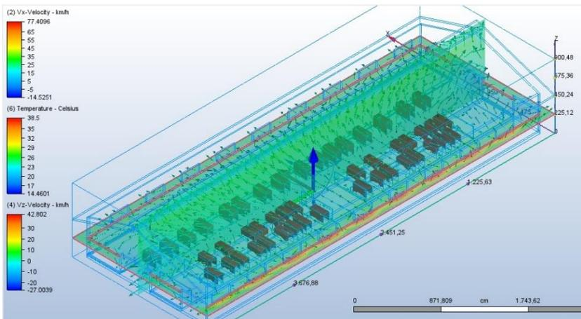
**Figure 22.** Autodesk CFD simulation of Study 2 data and movement of natural ventilation velocity in the vertical direction (z-axis)
