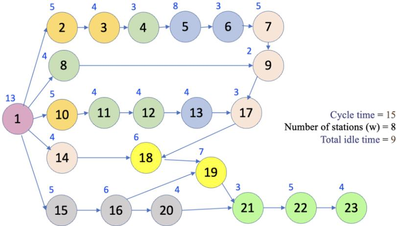
**Figure 3.** Precedence relationship graph with tasks color-coded by workstation allocation (CT=15).
