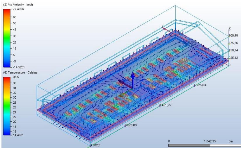
**Figure 20.** Autodesk CFD simulation of Study 2 temperature value and direction of movement
