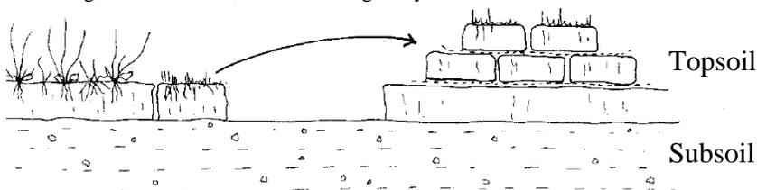
4. Re-lay level, without protruding edges. Fill the gaps with topsoil. Water well.
