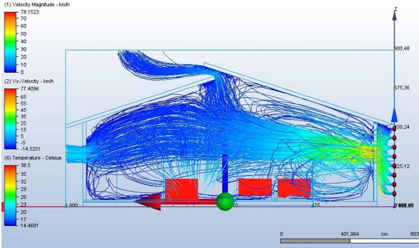
**Figure 25.** Autodesk CFD simulation of Study 2 natural ventilation movement 1
