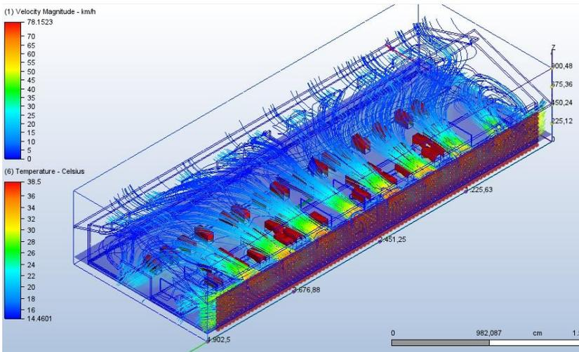
**Figure 24.** Autodesk CFD simulation of Study 2 temperature value and natural ventilation movement 1
