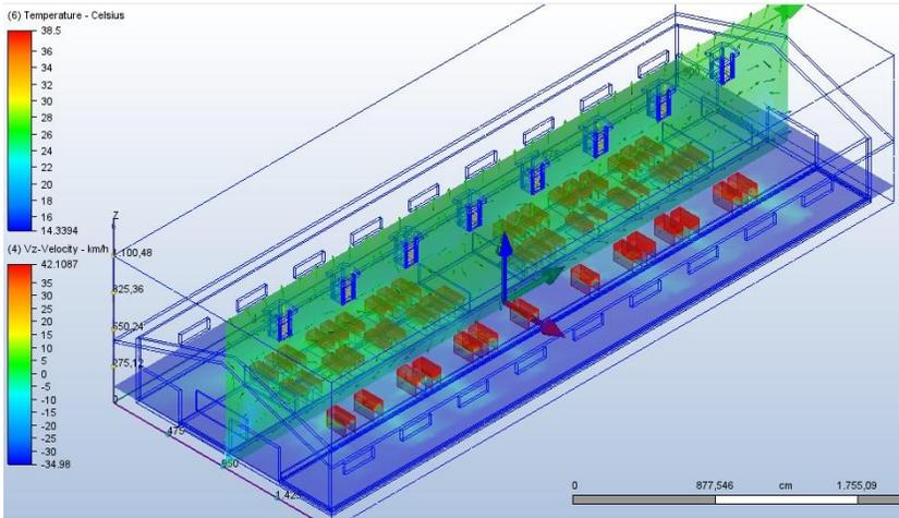
**Figure 15.** Autodesk CFD simulation of Study 1 data and movement of temperature value and natural ventilation rate in vertical direction (z-axis) at dairy cattle height
