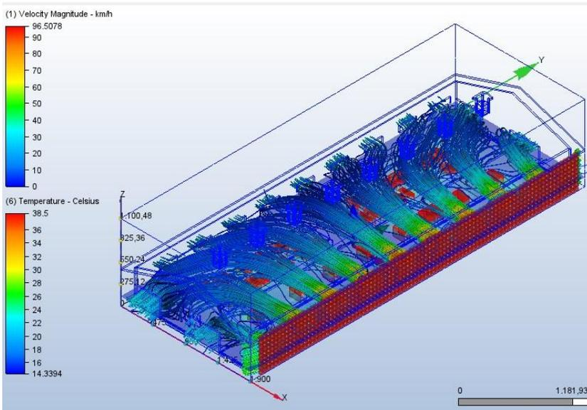
**Figure 16.** Autodesk CFD simulation temperature value and natural ventilation movement of Study 1
