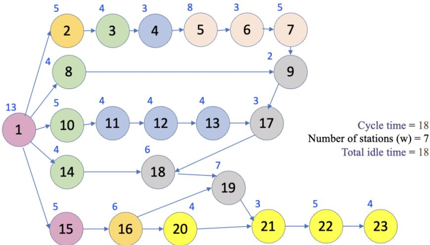
**Figure 3.** Precedence relationship graph with tasks color-coded by workstation allocation (CT=18).
