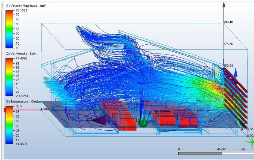
**Figure 26.** Autodesk CFD simulation of Study 2 natural ventilation movement 2
