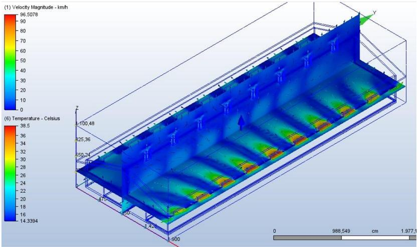
**Figure 13.** Autodesk CFD simulation natural ventilation movement velocity data for Study 1
