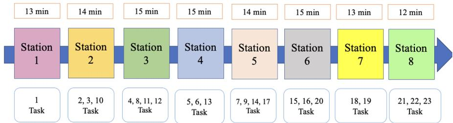
**Figure 4.** Flow diagram of 7 workstations with color-coded task allocation and processing times (CT=15).
