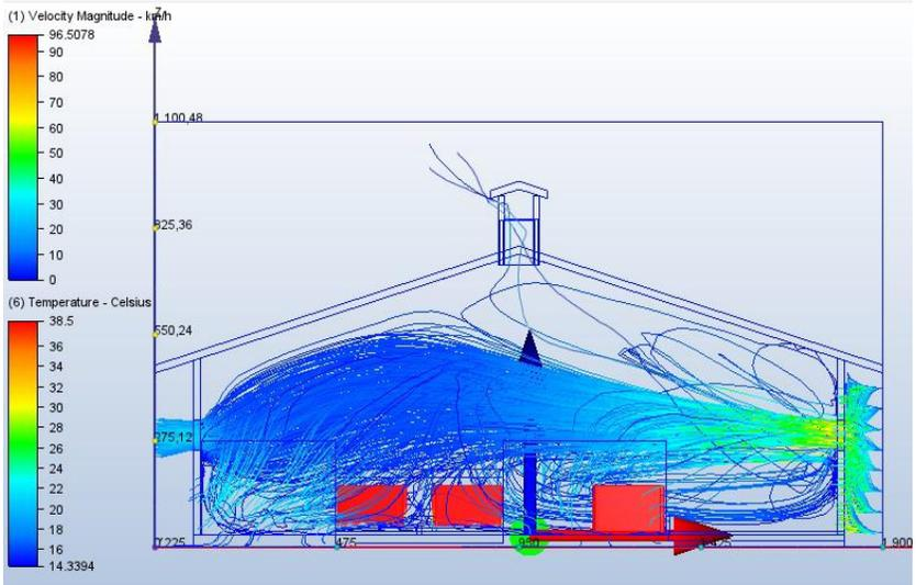
**Figure 17.** Autodesk CFD simulation of Study 1 natural ventilation movement 1
