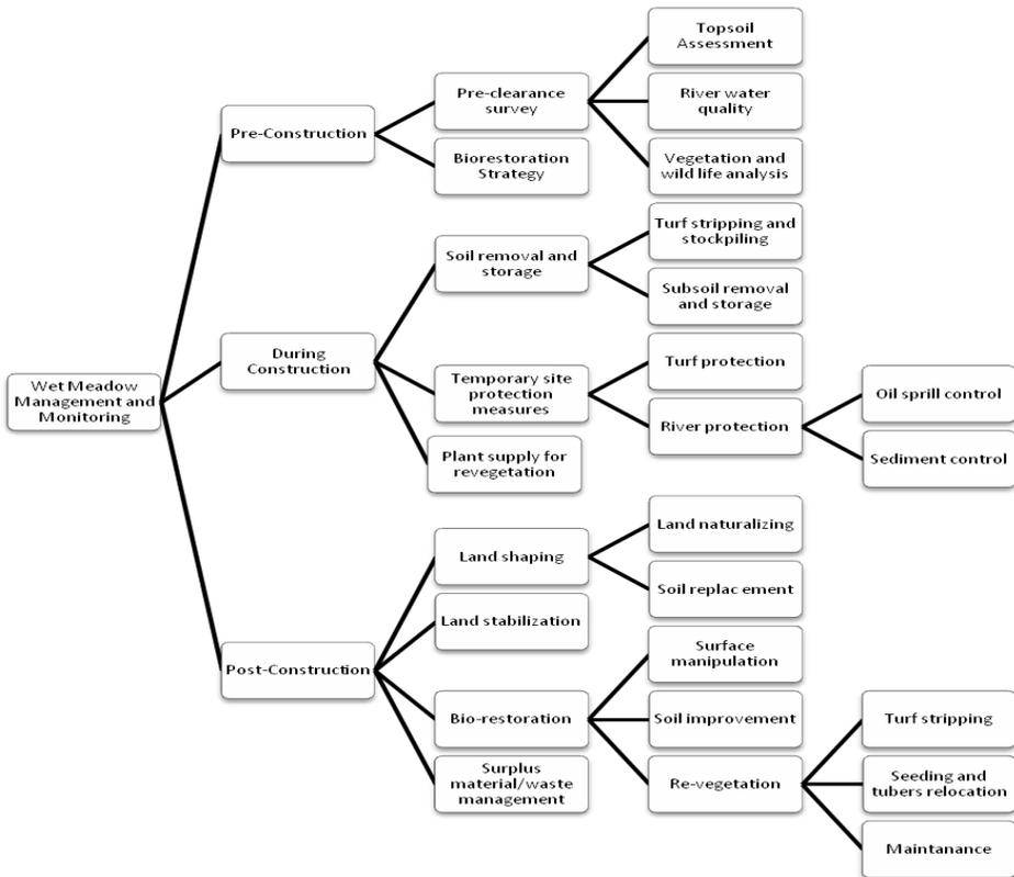
**Fig. 3** The components of reinstatement plan
