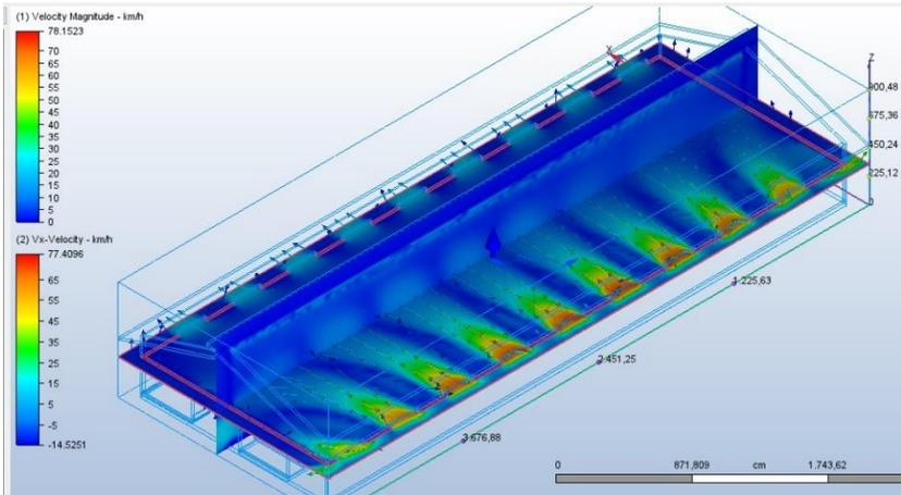
**Figure 21.** Autodesk CFD simulation natural ventilation movement velocity data for Study 2 1
