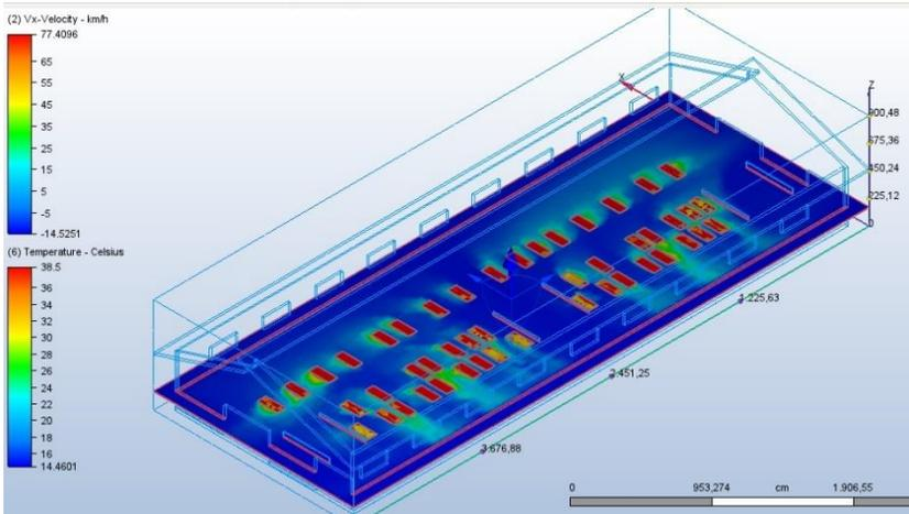
**Figure 19.** Autodesk CFD simulation temperature value of Study 2
