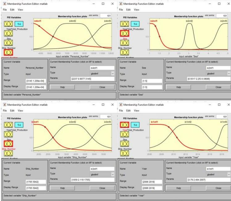
Figure 1. Membership functions of input variables for ANFIS model
