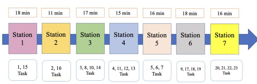
**Figure 4.** Flow diagram of 7 workstations with color-coded task allocation and processing times (CT=18).
