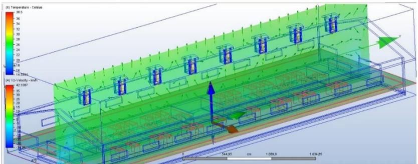
**Figure 14.** Data and movement of natural ventilation velocity in vertical direction (z-axis) in Autodesk CFD simulation of Study 1
