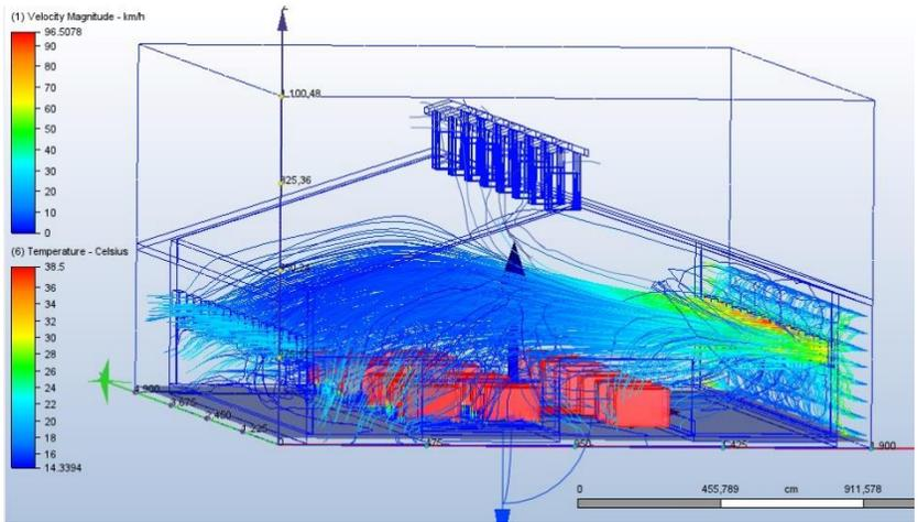
**Figure 18.** Autodesk CFD simulation of Study 1 natural ventilation movement 2
