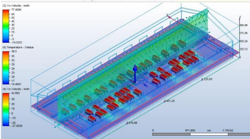
**Figure 23.** Autodesk CFD simulation of Study 2 data and movement of temperature value and natural ventilation rate in vertical direction (z-axis) at dairy cattle height
