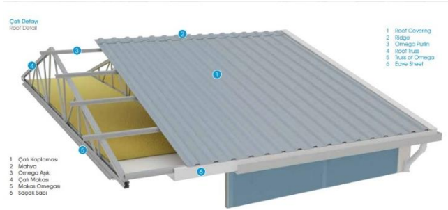
Figure 6. Roof Layers of Worker Barracks [8]
