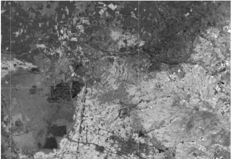
Figure 4.1 NDCI image showing chlorophyll-a values determined by scaling the bands of Sentinel 2 satellite imagery
