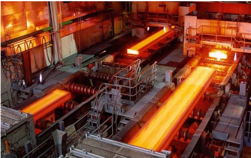
Figure 3. Production of armor steel by hot rolling.
