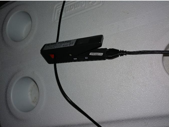
Show the clamp with the 10A setting.
