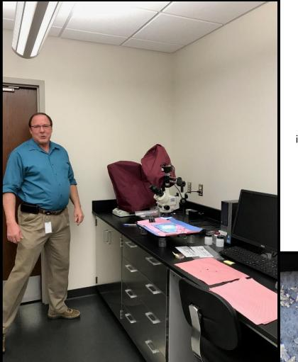
Dale Benson next to the inspection microscope looking at metal flakes in oil filters to visually identify the type of metal and determine the component that is wearing.
