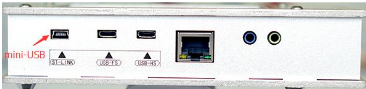
Picture 2: Powering the Unit Up from ST-LINK Port
