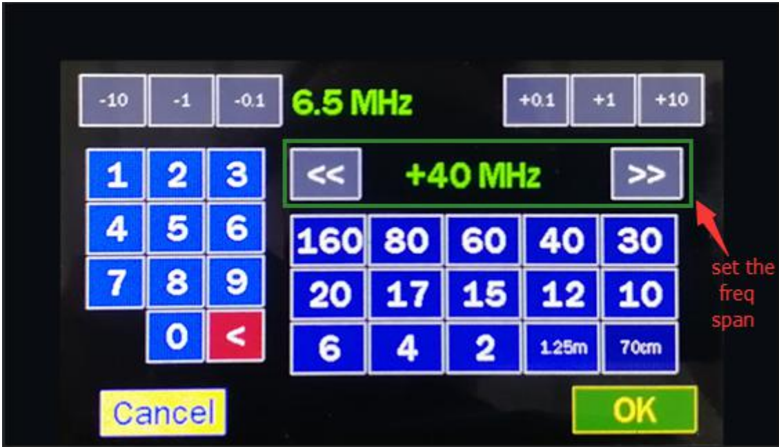
Picture 22: Setting span in panoramic scan
