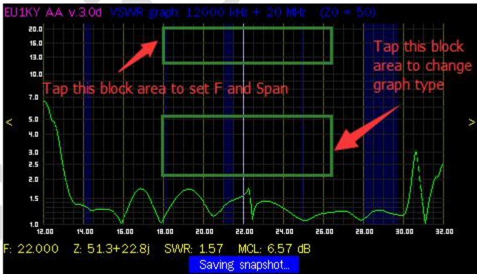
Picture 19: Changing frequency and graph switching in panoramic scan
