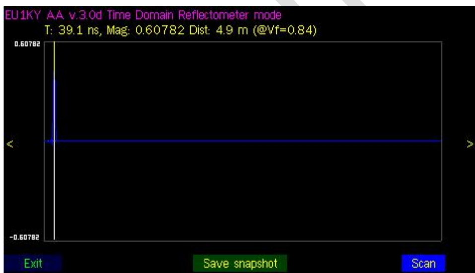
Picture 30: Moving the maker to the peak to find the distance
