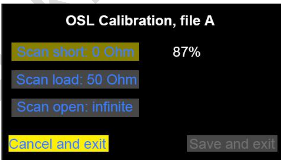
Picture 34: Scanning 0 Ohm load is in progress
