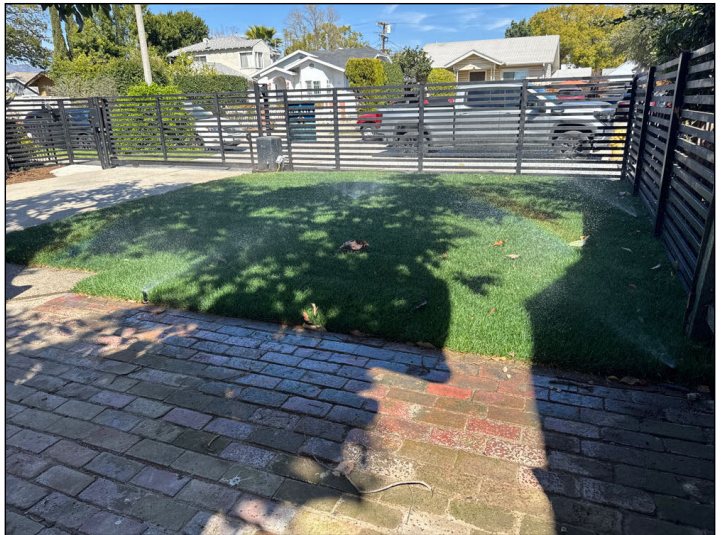
Adjust spray away from structures, sidewalks or fences to prevent moisture penetration and damage.
