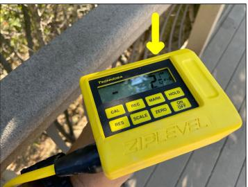
Significant settlement within a 10 foot span.
