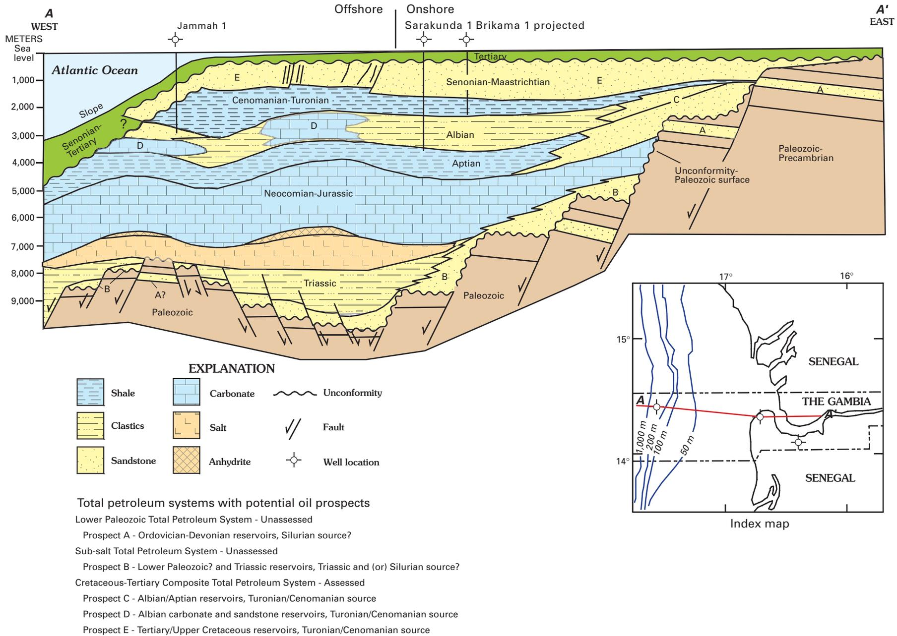
**Figure 9.** Schematic east-to-west cross section through The Gambia showing locations of potential oil prospects with their associated total petroleum systems, reservoirs, and source rocks. Modified from Bungener (1995).
