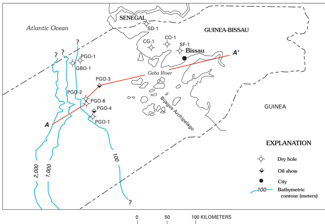
**Figure 5.** Location map for Guinea-Bissau showing line of section and oil and gas exploration holes, southern Senegal Basin, northwest Africa. Cross section A to A' is shown in figure 6. Modified from Dumestre and Carvalho (1985).
