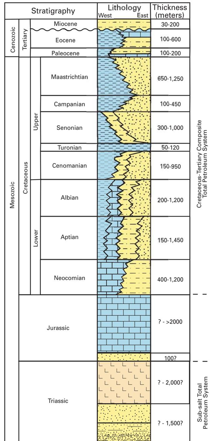
**Figure 8.** Generalized stratigraphic column for the Northern subs basin and the southern part of the Mauritania subbasins (see fig. 3). Type II and III source rocks are found in the Cenomanian and Turonian units. Modified from Dumestre (1985).
