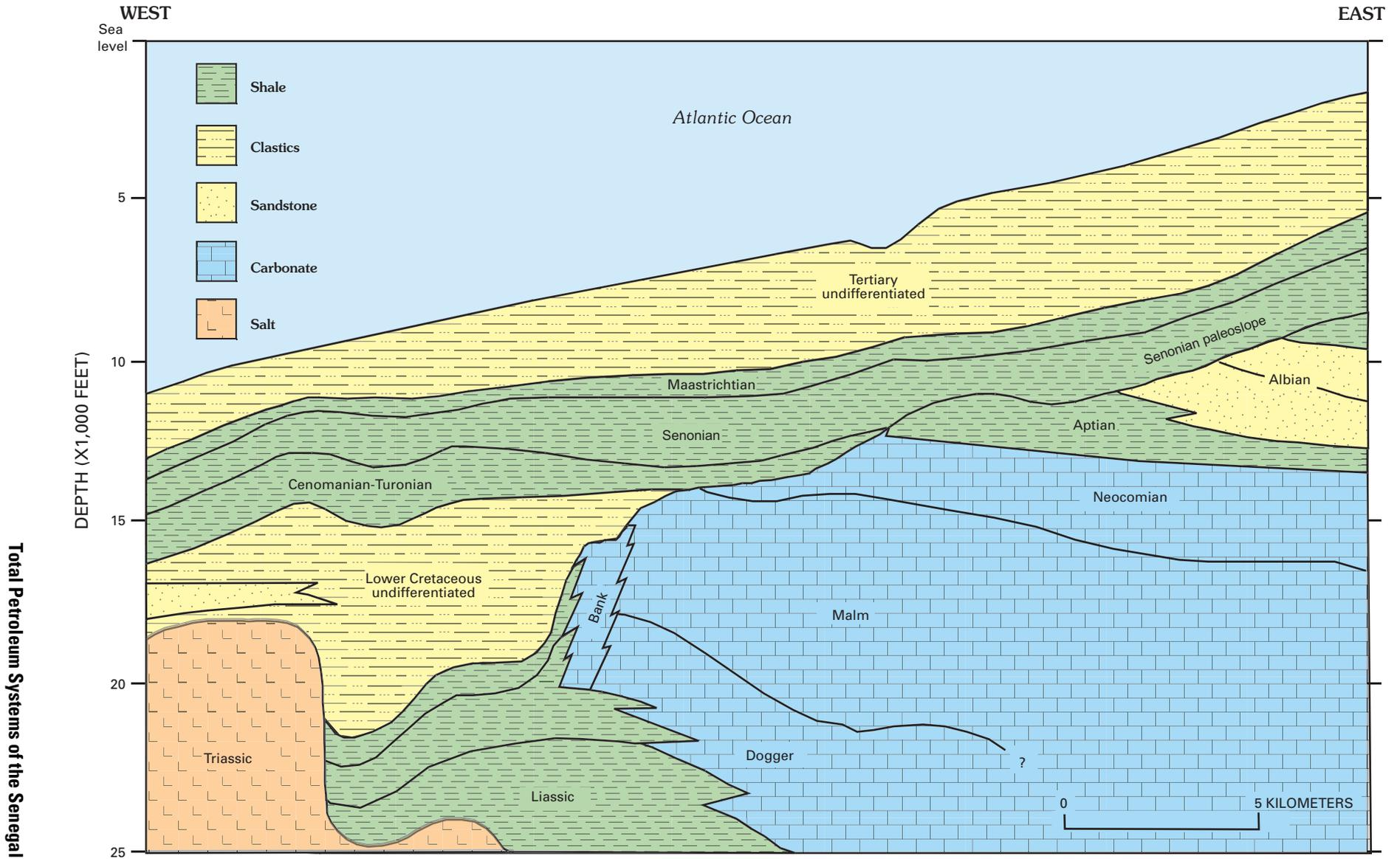
**Figure 18.** Schematic cross section of offshore Guinea-Bissau, Senegal Basin, northwest Africa. The Albian-Cenomanian Geba delta prograded westward across the carbonate platform providing reservoir-potential sands and source rocks. The carbonate and deltaic rocks subcrop the Senonian paleoslope, offering several areas of potential traps. Modified from Clifford (1986).
