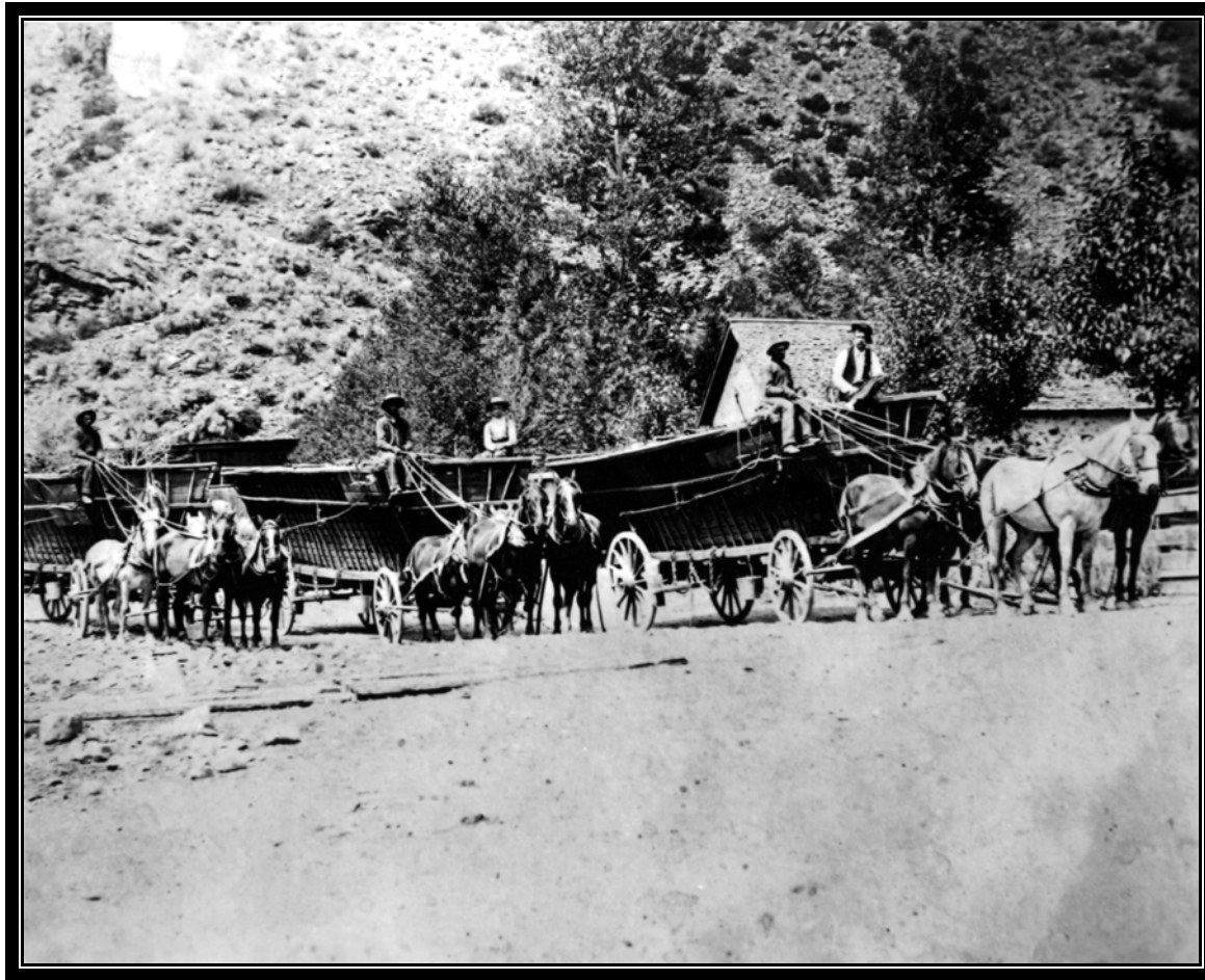
Figure 7. Coke wagon used to transport charcoal to the Clayton smelter, c. 1912. Photograph used courtesy of Clayton Area Historical Association ( www.claytonidaho.org ).
