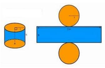
This is what is meant by surface area. This is the view if we unroll the cylinder, and add the top and bottom of the cylinder
