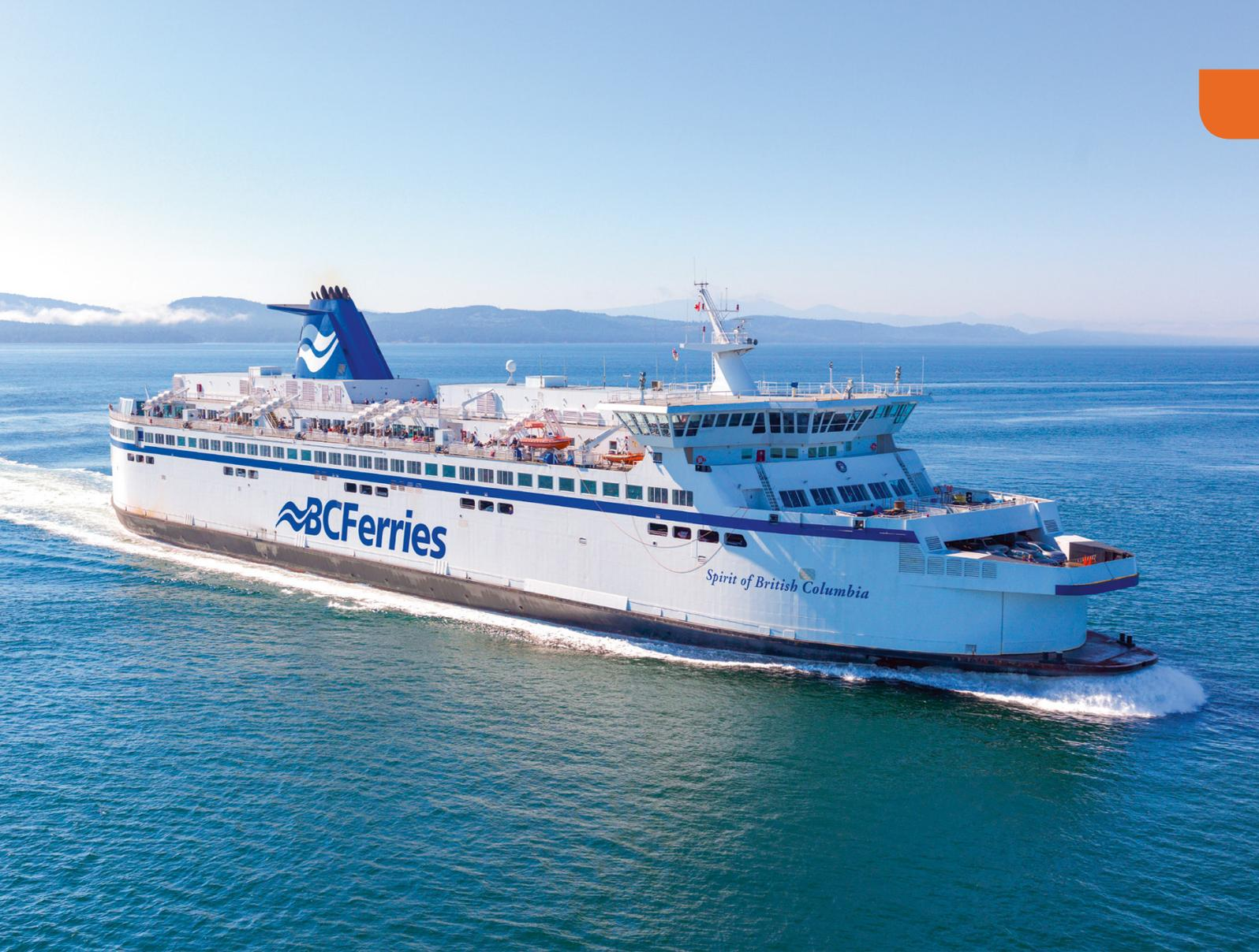
BC Ferries' Spirit of British Columbia was recently retrofitted with dual-fuel engines to allow her to operate on cleaner natural gas
