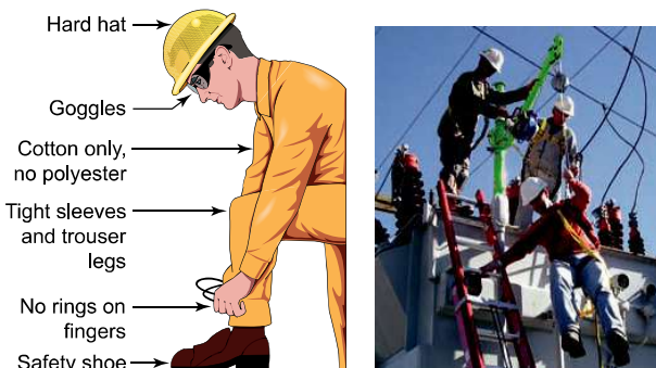
Figure 1-4 Appropriate attire should be worn for each particular job site and work activity.
