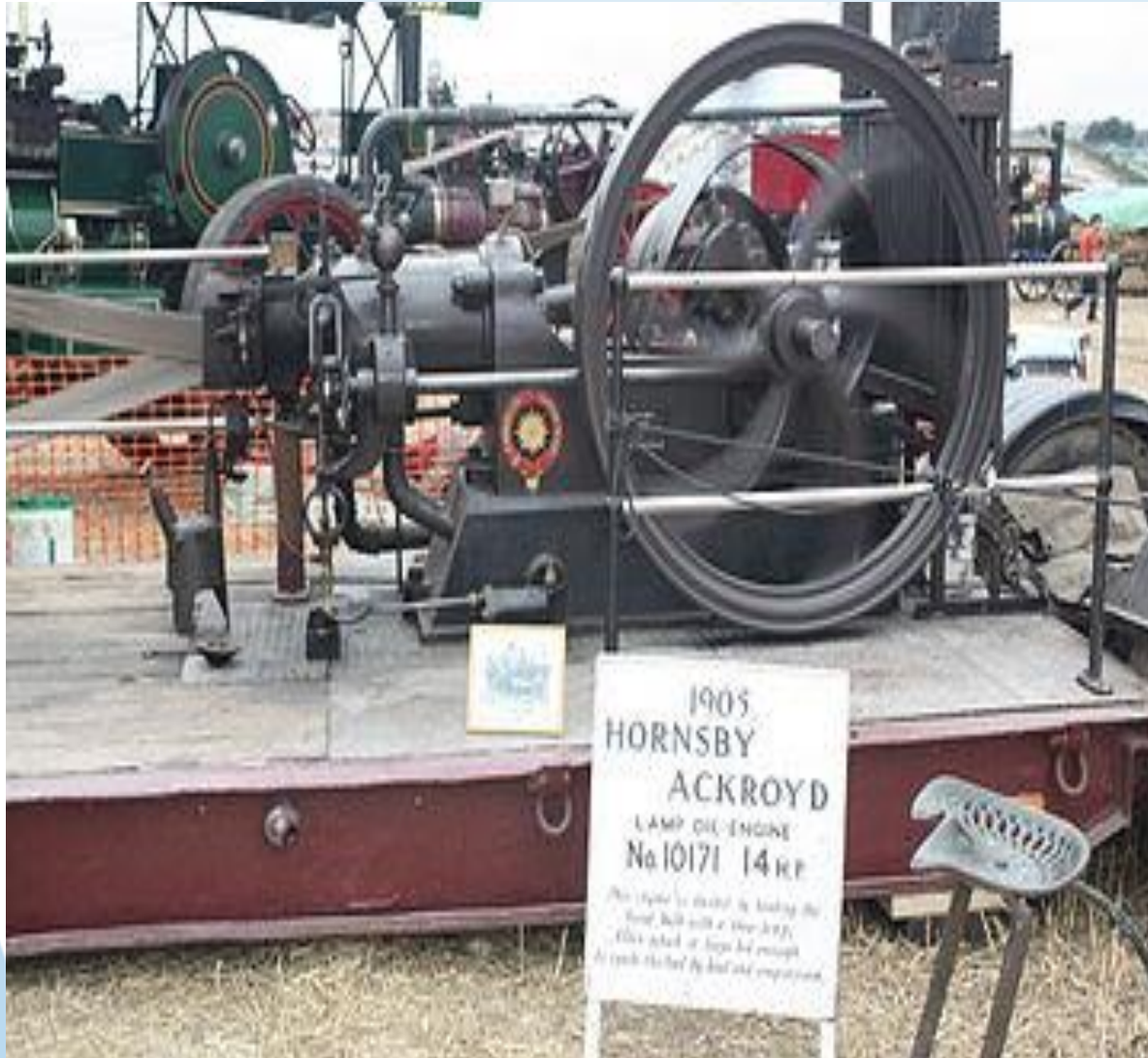
Hornsby- Akroyd oil engine (1905): Four-stroke, 14 HP
