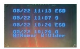
The PUMP RECORD screen can be accessed from the main menu by pressing \*. You can also access this screen directly when POC is in sleep mode by pressing \*, skipping the MAIN MENU screen. When in the PUMP RECORD screen, pressing A or B will scroll through the pump records. The most recent 100 pump records are retained.
