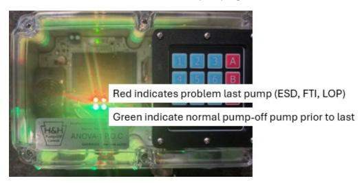
The STATUS LEDs are a shortcut to see the status of a well without the need to get out of vehicle and wake up the POC. Each row of lights is treated as a single message and are always the same color. In general, the top row corresponds to the last pump, and the bottom row indicates the status of the pump prior to the last. Green lights indicate normal pump-off. TO and LT are indicated by yellow lights. FTI, ESD or LOP are indicated by red lights.
