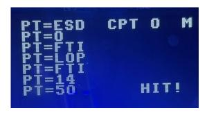
When the POC has a command either from a timer or from the user to pump the well, it will first give a warning screen and beep for several seconds, then start the well. It will then rapidly move through FTI and ACTIVE LEARN screens. Once the PUMP SCREEN is shown, the POC is working to detect pump-off.
