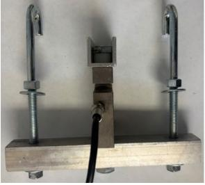
Assemble the harness on the sensor as shown. Use long bolt on square bar side and short bolt and nylon washer on C-channel side. The C-channel does not have to be tight, twist until tight then back off so that channel is aligned with sensor as shown.
