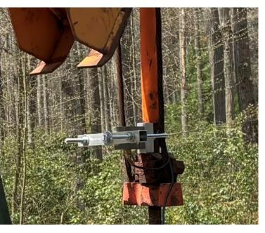
To mount harness to well, rest C-channel on top of the polish rod clamp and against polish rod. Hook J-bolts around bridle cables and tighten nuts by hand to keep in place. J-bolts can be turned inward for smaller carrier bars, or outward for larger bars.
