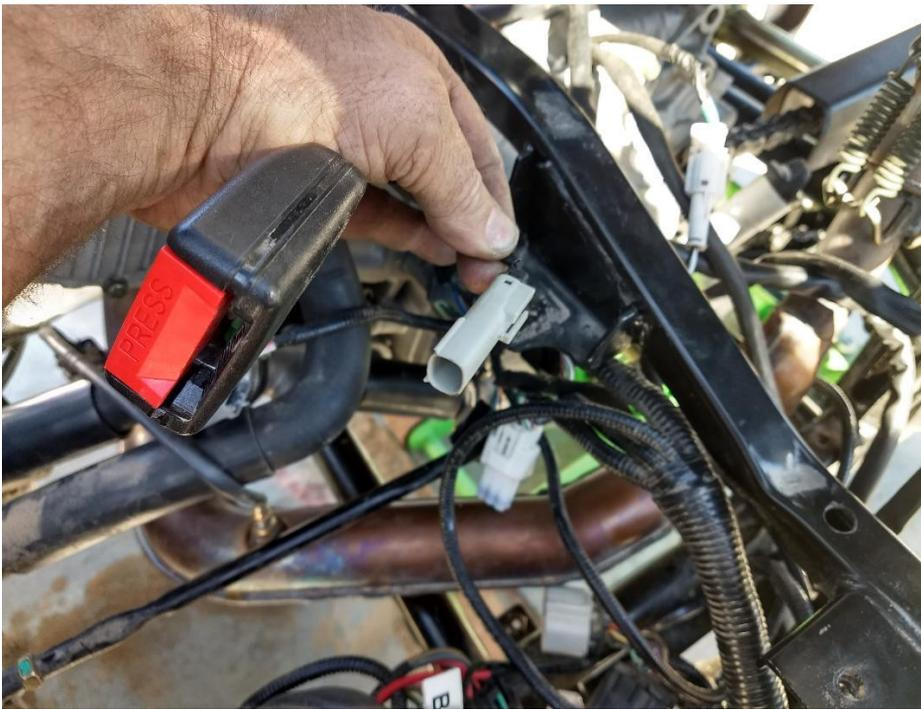
Again, If this plug is disconnected it will think it the seat belt is plugged in and not have any speed restriction.
