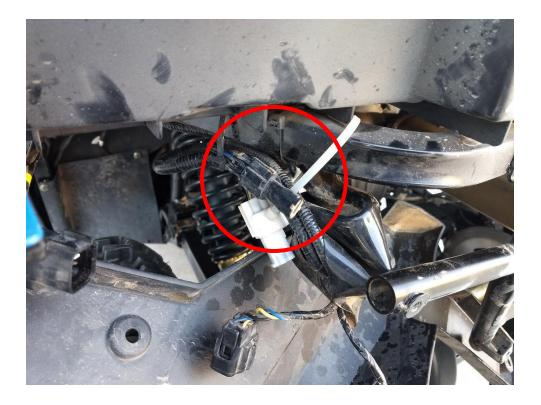
The next upgrade is another item you might never realize, but it has been upgraded. The fuel tank has a new design, this includes a new fuel pump and connectors. The new tanks uses a feed and return line to the pump. It also has a vent line to the emission canister. Strike and Sector models.
