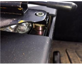
HiSUN had to meet the new emission standards on the Strike and Sector and one of the things they added was a new emission canister. It is located behind the passenger on the right side by the VIN tag. Do not remove this please, it will not give you any more power without it. Strike and Sector models.
