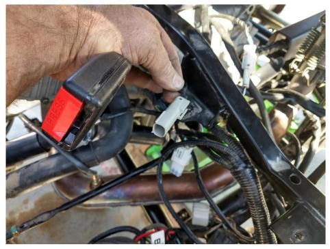
Again, If this plug is disconnected it will think it the seat belt is plugged in and not have any speed restriction.
