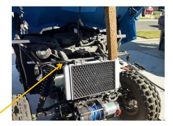
You might also have to crack open one of the small 8mm bolts in the cylinder head to allow some air pressure escape as well.
