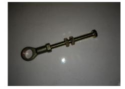
Next is to remove the long bolt from the adjusting mount. Remove the nuts from the long bolt and set aside. Place a small amount of blue loctite on the threads on the long bolt and re-insert into the adjusting mount until it stops.
