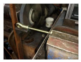
Next is to clean up the end of the bolt you just cut so that you can re-install one of the nuts that you removed originally. Tighten the nut at the end of the adjusting mount snug Next is to install a strong and thick washer like the one shown in pic 4 along with a 8x1.25 nylon lock nut.
