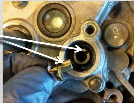
When removing the left side cover, it is **not** necessary to remove this bolt. It is a coolant bleed hole and has an aluminum washer behind it.
