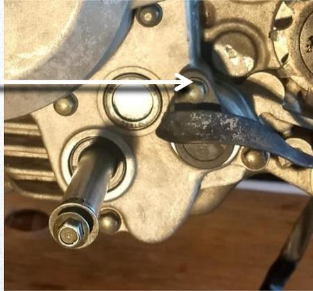
Inspect the switch for corrosion and or damage. If the contacts appear dirty, clean them with some 3M scotchbrite pads lightly.
