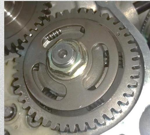
3. Install the outer locking plate balance gear and torque the 19mm nut down to 61 ft. lbs
