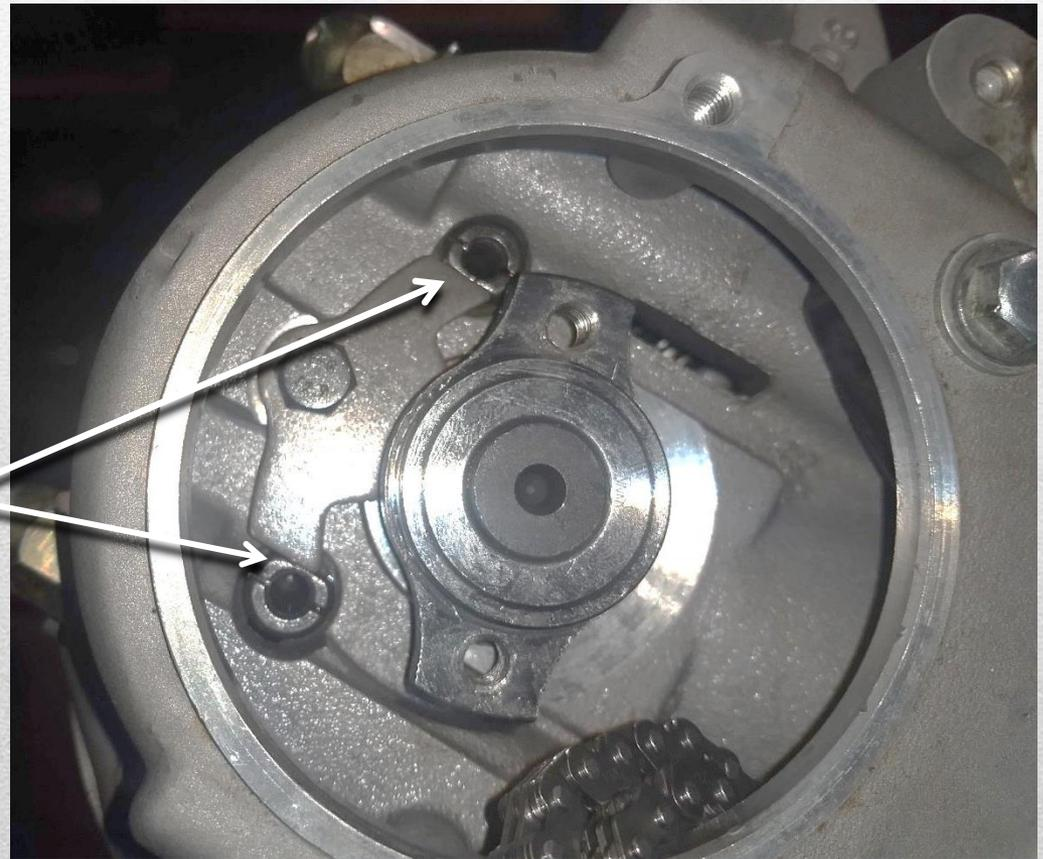
Inspection port for valve adjustments.
