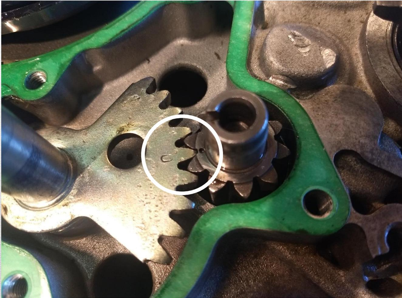
With the flywheel removed you can see the proper way the starter gear and starter idler gear are placed. This gear only turns one way due to the one way bearing on the opposite side.
