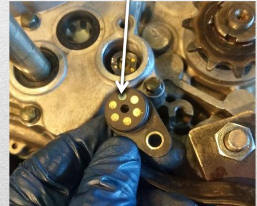
Inside you will find a metal pin. This contacts the switch and tells the computer what gear the UTV is in
