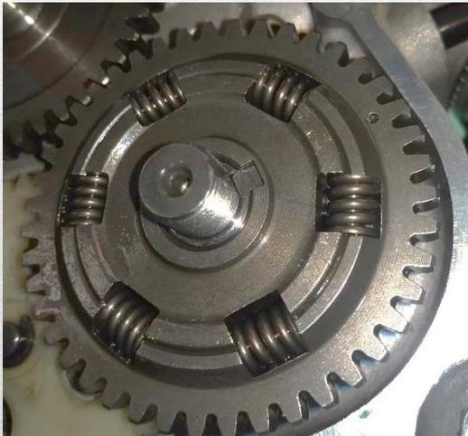
2. Install the balance drive gear assembly next making sure to install the key way here.
