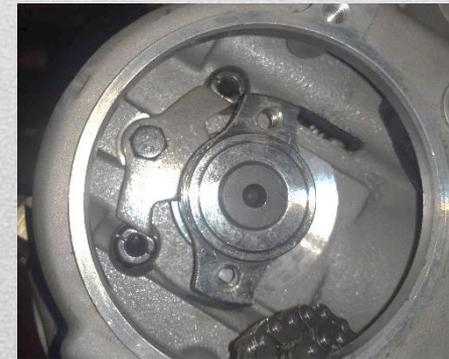
Install the cam gear with the cam chain so that it is aligned with the marks on the cylinder head. Making sure the engine is Top Dead Center.
