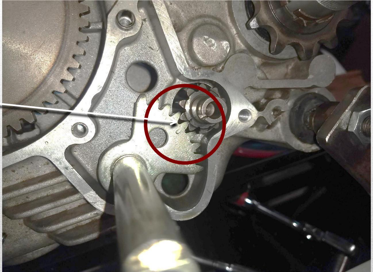
1. Install the locking plate balance gear against the gear on the balance shaft
