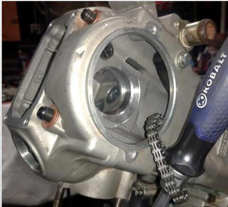
Here something is used to help hold tension on the cam chain while the cylinder head is mounted. Torque the main head nuts down to 26 ft. lbs.
