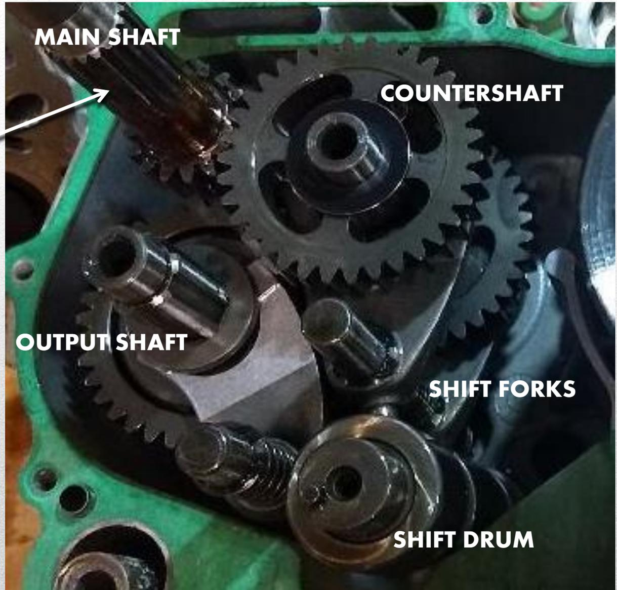
Installation of the transmission is a little tricky. The countershaft assembly and the output shaft need to be installed along with the shift forks at the same time to make installation simple. It can be done separate but might take some time to align the gears. *We have a video on our website to show how to correctly install the transmission. As well as on YouTube: Hisun 250 Transmission installation.*
