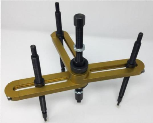
**CASE SPLITTER TOOL** (I got mine from factory wrench tools)
