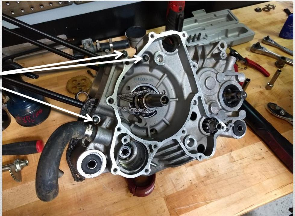
On the right side of the engine, remove the remaining 8mm bolts that connect the case halves together.
