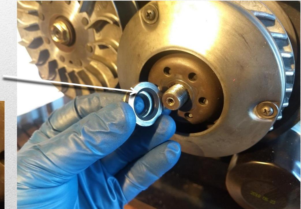
Next is to remove the Variator and set aside. You will now be ready to remove the main clutch assembly. Use 2 of the 10mm bolts that held the clutch plastic cover on and you will use them to help push the clutch open to aid in removing the CVT belt.
