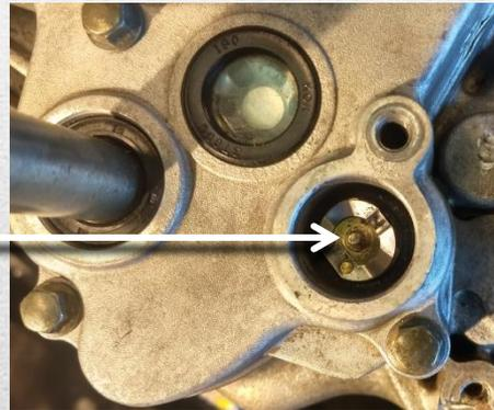
Pull the switch tab out of the hole and set aside. Take note to see the tab on the side of the pin and the slot on the shift drum
