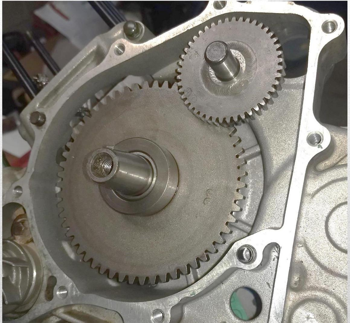
Install the fan shift gear assembly. (shift rod) into the case as in the picture below. Making sure the mark on the shaft aligns with the dot on the shift drum.
