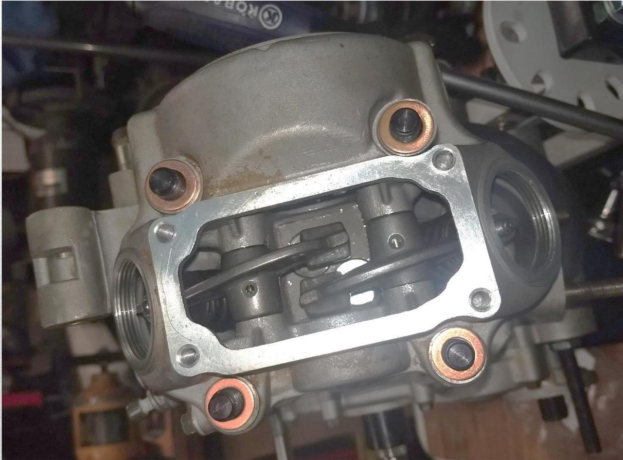
Here you can see the cam retaining plate. The rocker shafts are installed so that the flat side to the shafts rest against the retaining plate, securing them in place. Remove the bolt holding the plate in place. You can now remove the cam if the rocker adjustments are loose enough.
