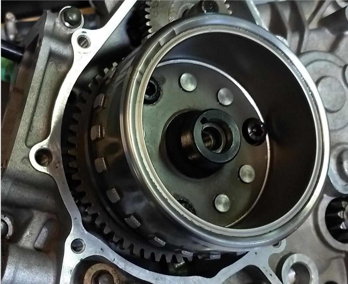
Install the left side magneto cover at this time. Torque the 8mm bolts down to 8.5-9 ft. lbs.
