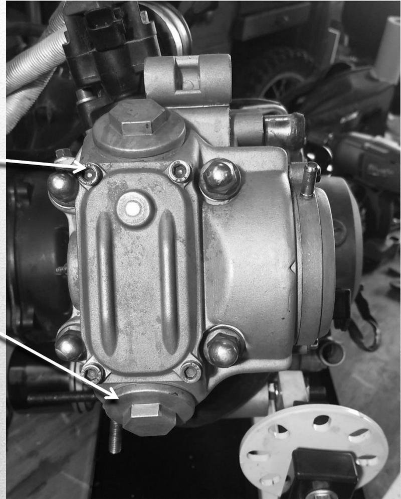
Remove the side cover on the cylinder head to access the cam gear and timing chain. Remove the cam chain tensioner first, then remove the 2 bolts holding the cam gear to the cam. Then move the gear out and place aside. Try to hold the cam chain secure with wire or another means to prevent it from falling into the engine.
