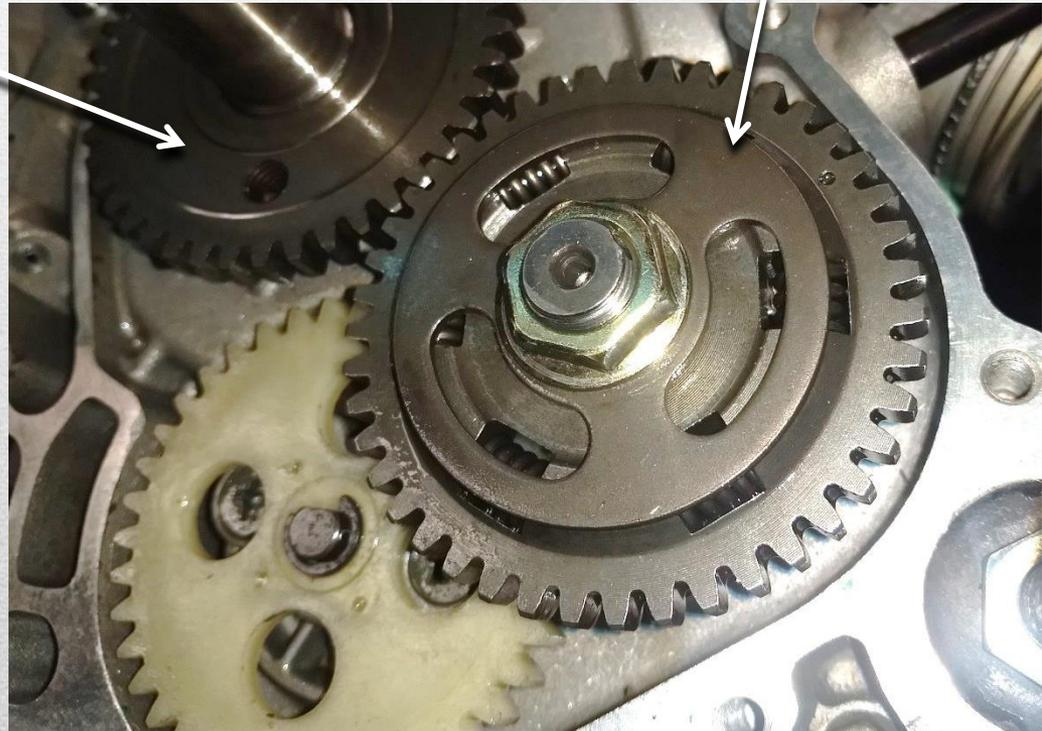
Next is to remove the oil pump. You will need to use a impact driver tool to assist without damaging the 2 screws. We stock high quality replacement screws
