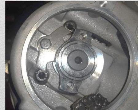
Install the cam gear with the cam chain so that it is aligned with the marks on the cylinder head. Making sure the engine is Top Dead Center.
