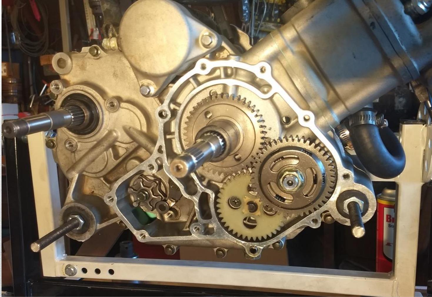
Here is the timing mark for the crank and counter balance shaft. Ensure these marks line up when re-installing the parts. Failure to do so can cause engine running problems and possibly engine failure. **When install the cases together it is important to turn the balance shaft a bit to ensure the gears on the opposite side align with the water pump gear. Failure to do so might cause the balance shaft to bind and not rotate or damage the water pump gear.**
