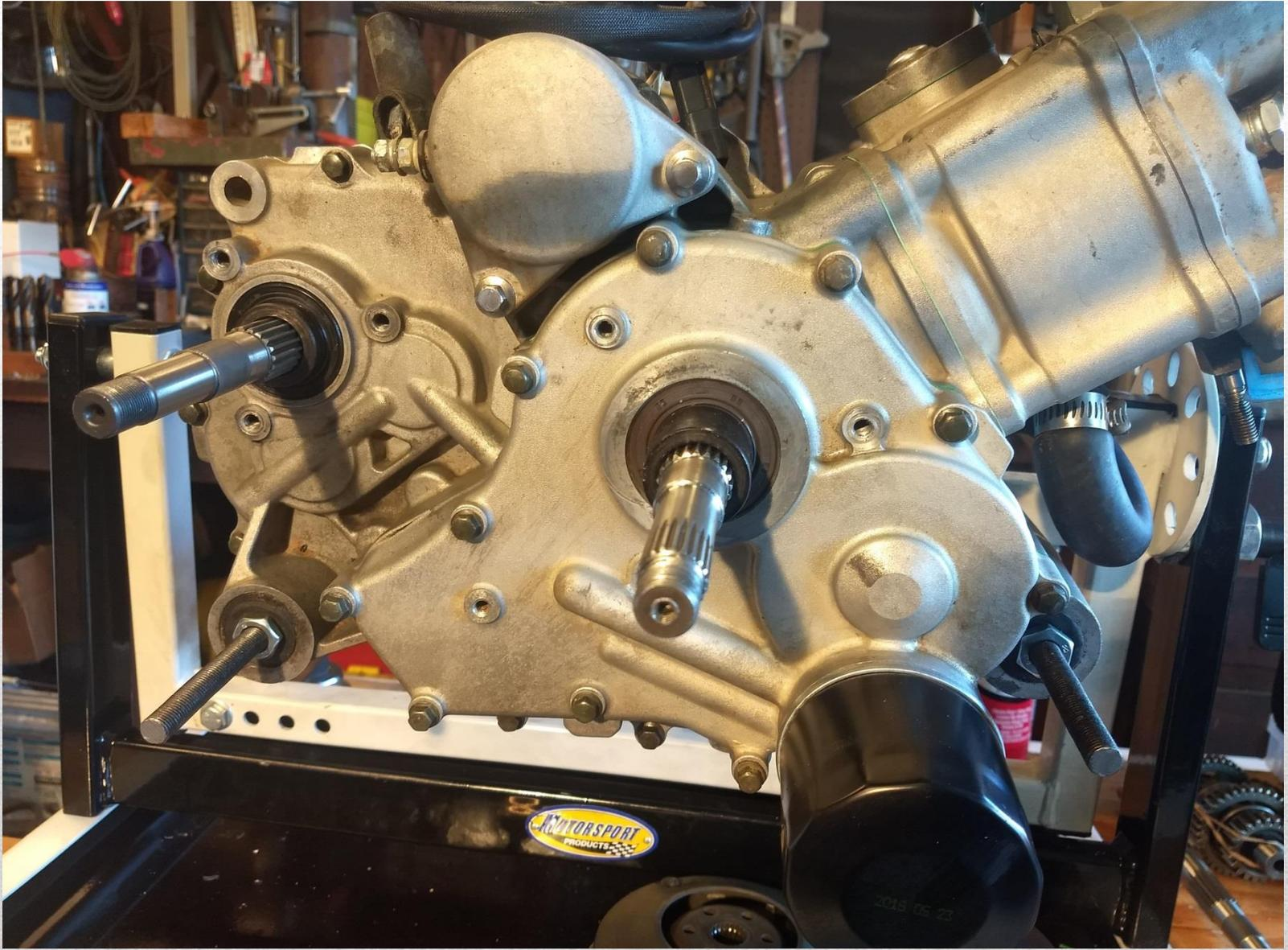
To remove the right side cover, there is a hidden bolt behind the oil filter. Remove the oil filter and locate the allen head bolt. Remove this bolt along with the remaining 8mm hex head bolts securing the side cover on. Pull straight off of the shaft. When re installing this bolt, tighten to 8.5-9 ft lbs.
