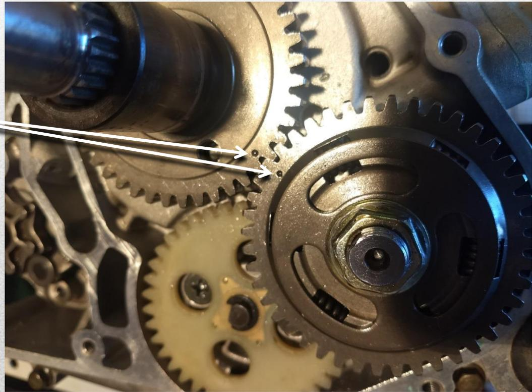
To remove the left side cover, start by removing the bolt and washer on the shift shaft. (c) This bolt and washer will prevent the side cover from fully being removed and possibly damage the seal.
