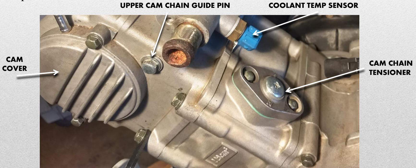
Final assembly should be in the order removed.
