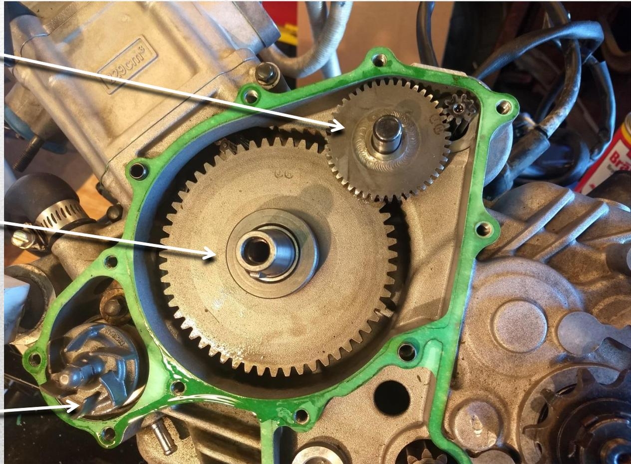
Pull the starter gear and starter idler gear out and place aside. Next is to remove the countershaft sprocket. Using a special socket.
