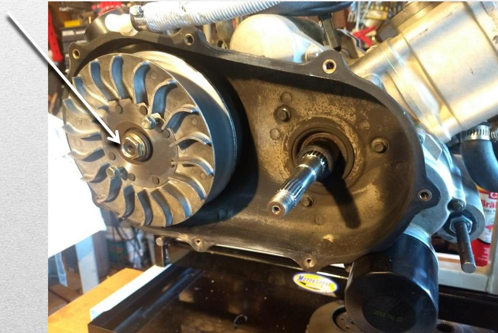
Here you should see the clutch bell along with a special sized washer. This washer rides on the bearing in the clutch assembly and correctly spaces out the clutch bell from the clutch.
