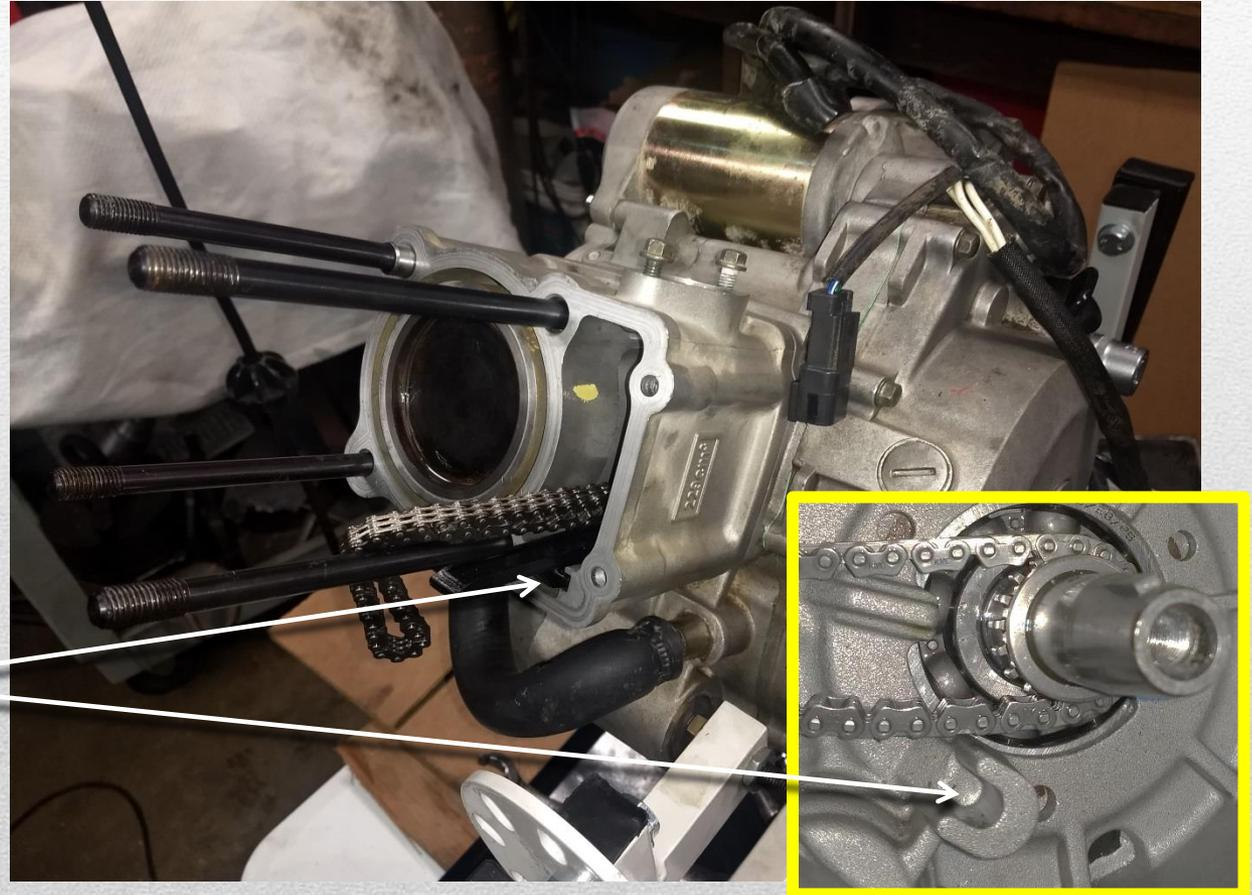
Place the cylinder head on top of the engine. Using a new head gasket. Place the head with the cam chain guide inside the head and pull the cam chain through the cam side opening. Secure the chain so that it will not fall down into the engine, keeping tension on the chain to prevent it from coming off the gear on the crankshaft below.
