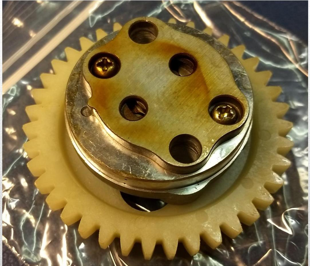
Install the balance gear on the crankshaft at this point. With the shoulder side facing the engine. Ensure the key way is installed as well
