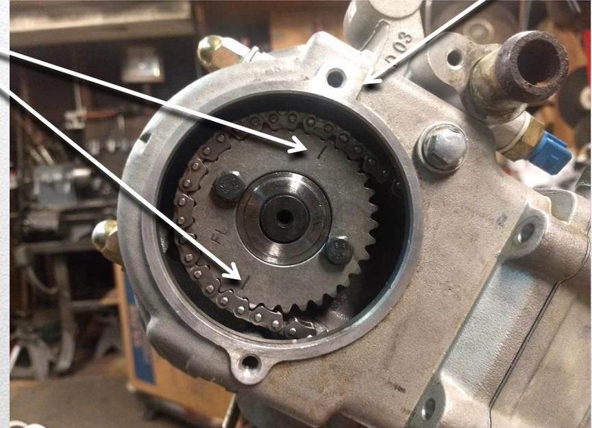
T timing mark showing through the viewing port on the stator cover.
