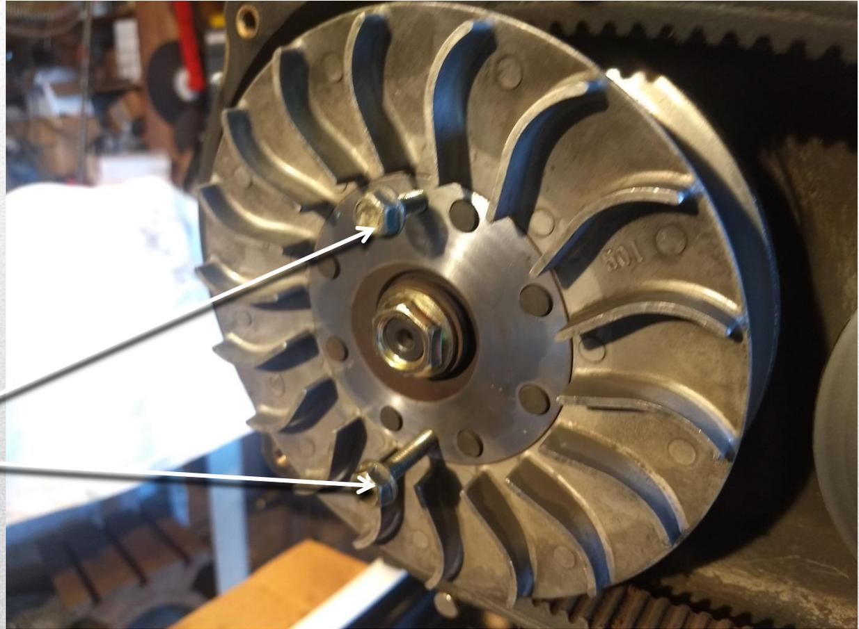
Once the CVT belt is removed, you will now remove the rear sheave behind the variator.
