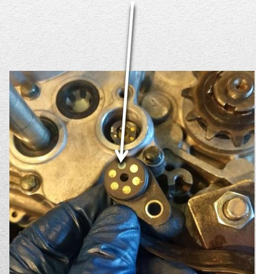
Inside you will find a metal pin. This contacts the switch and tells the computer what gear the UTV is in
