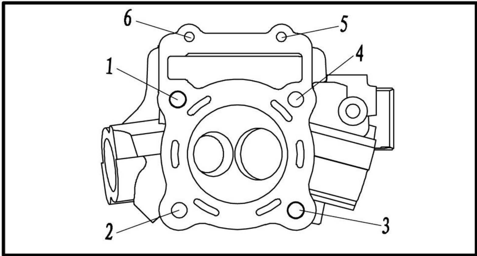
View of the cylinder head with the cover removed and the head nuts removed. *Always use new copper washers when installing the head.*
