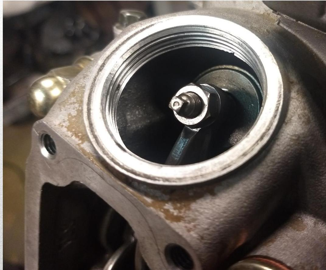
With the cylinder head pulled off, you can slide the cylinder up and off. Next is to remove the cam chain off the crank gear.
