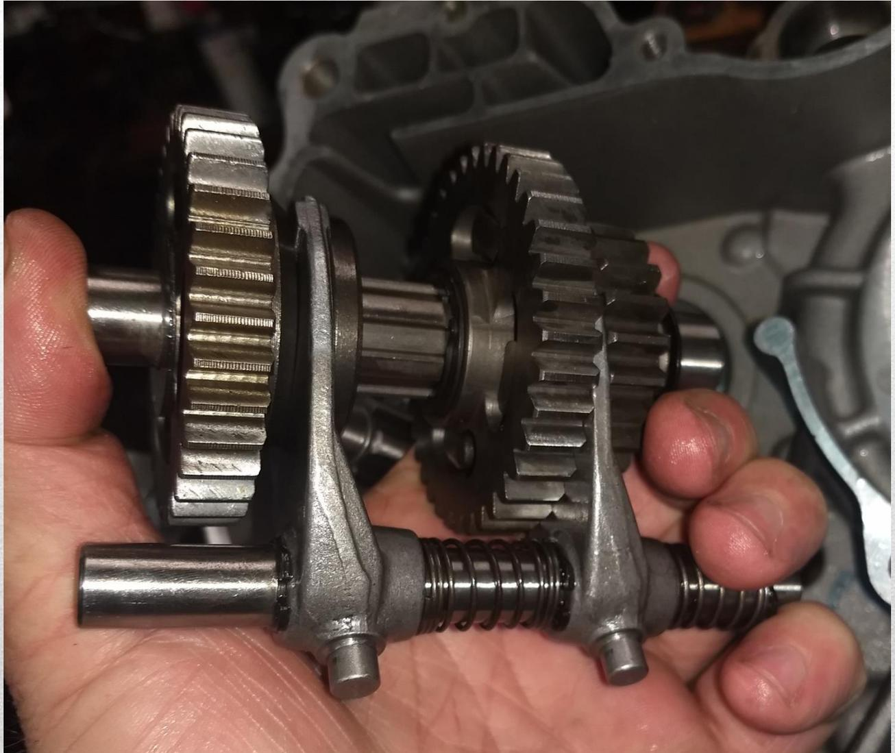
Installation can be tricky, try to install the transmission parts as complete as possible for alignment issues. The main shaft can be installed last as it has no alignment problem.
