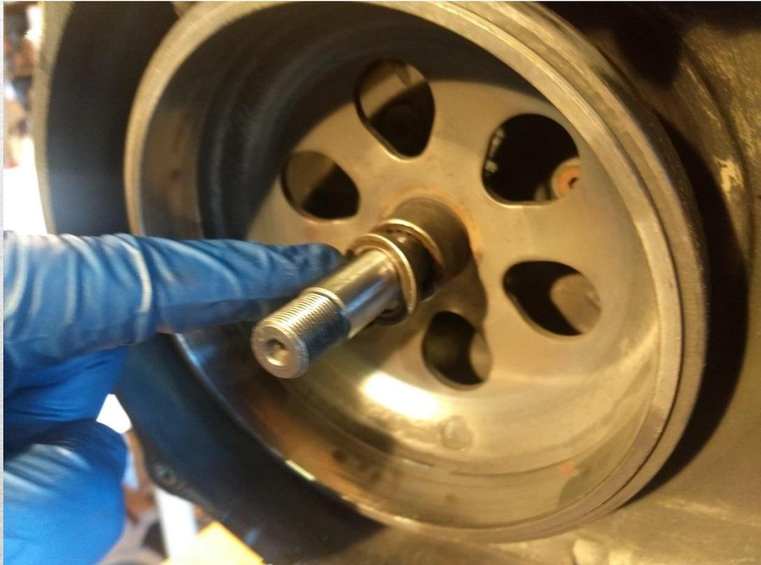
Here is the clutch housing. There are 6 bolts total securing it to the engine. Remove the 3 screws behind the clutch, and the 3 bolts behind the Variator.
