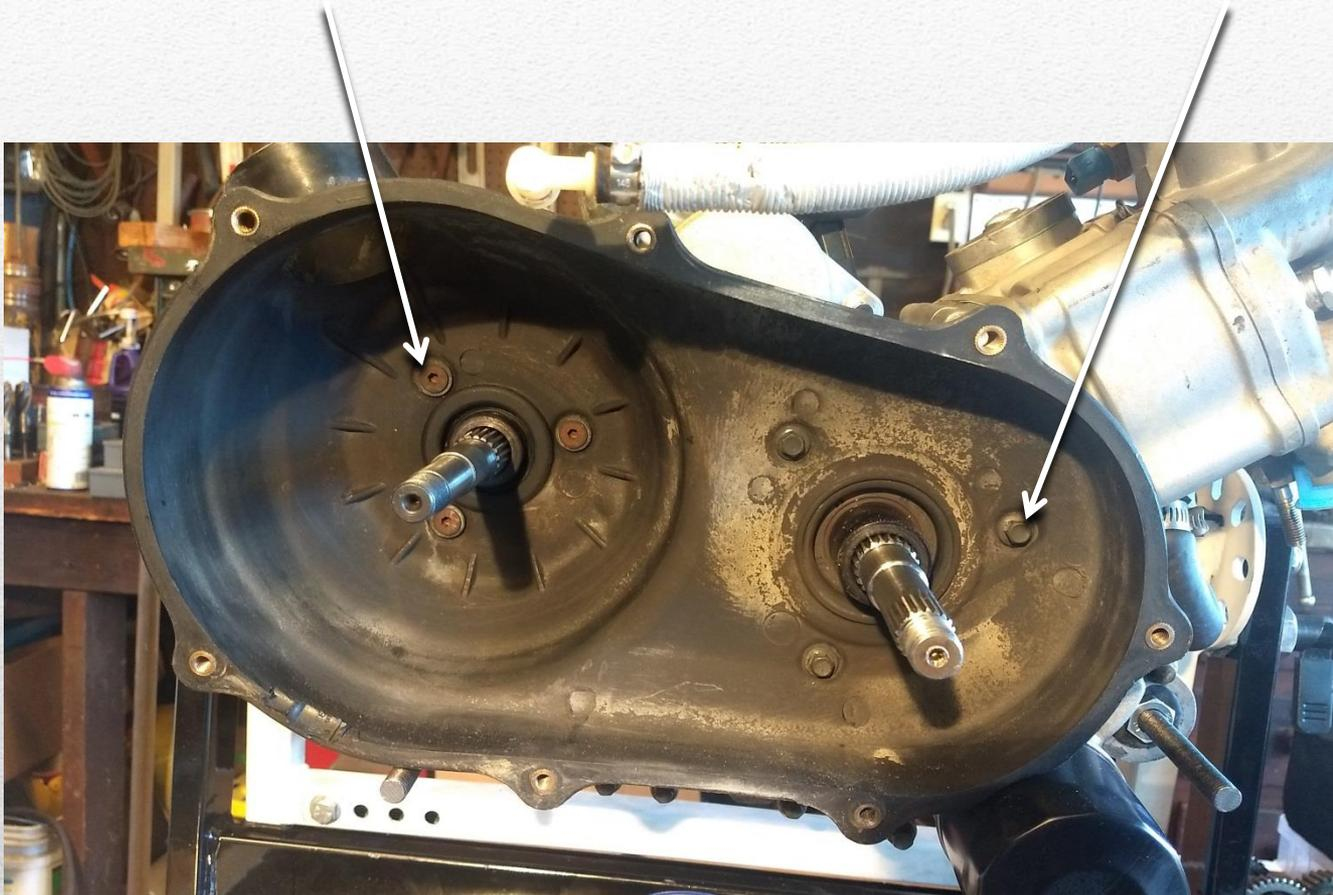
Use blue loctite when re installing as they can come loose and cause damage
