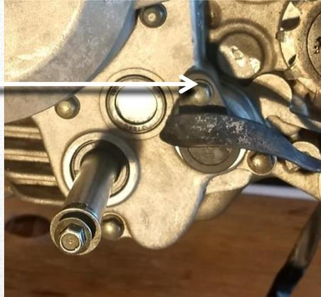
Inspect the switch for corrosion and or damage. If the contacts appear dirty, clean them with some 3M scotchbrite pads lightly.
