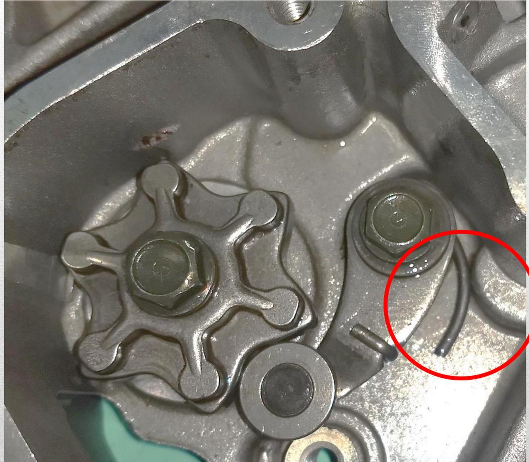
Install the cam chain on the crankshaft gear on the left side of the engine. Pull the chain through the opening in the case half.
