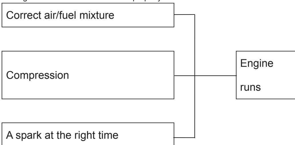
If one basic requirement is missing the engine will not run.
