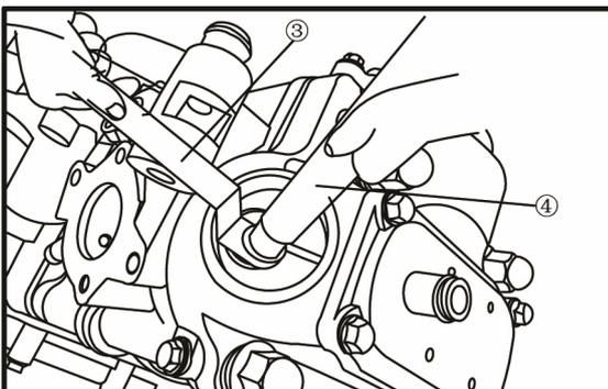
4. Adjust the valve clearance of cylinder .
