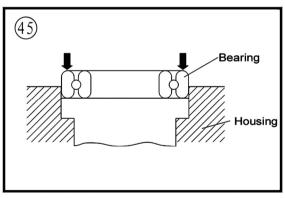
make sure to support both bearing races with wooden blocks as shown.
