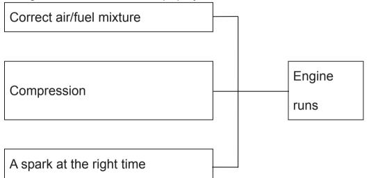
If one basic requirement is missing the engine will not run.
