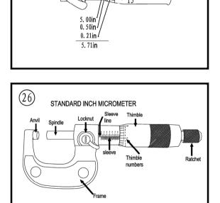
of the thimble aligns its 0 mark with the first line lower half of the sleeve line or 0.50mm.
