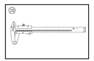
Properly maintain the measuring surfaces of the caliper. There must not be any dirt or burrs between the tool and the object being measured. Never force the caliper to close around an object. Close the caliper around the highest point so it can be removed with a slight drag. Some calipers require calibration. Always refer to the manufacturer's instructions when using a new or unfamiliar caliper.
