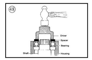
the balls will push against the outer bearing race and damage it
