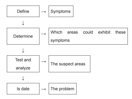
By following a systematic approach, the possibility of unnecessary parts replacement can be avoid, always start with the simple and most obvious checks when troubleshooting, This would include
