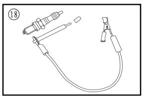
Make the tool shown from a No.6 screw and nut,
