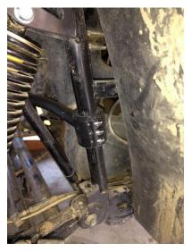
Do not tighten the Allen bolts until they are all started evenly. You will still be able to gain access to the air filter with this hitch.
