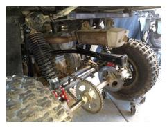
Mount on each frame rail with the supplied Allen wrench as high as possible to ensure the chain doesn't rub the hitch
