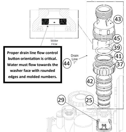
Proper drain line flow control button orientation is critical. Water must flow towards the washer face with rounded edges and molded numbers.
