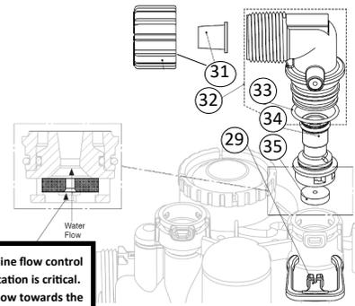
Proper drain line flow control button orientation is critical. Water must flow towards the washer face with rounded edges and molded numbers.
