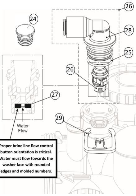
Proper brine line flow control button orientation is critical. Water must flow towards the washer face with rounded edges and molded numbers.
