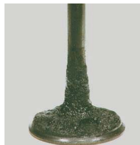
Picture D - Intake valve before P.i. treatment
