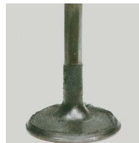
Picture E - Intake valve after P.i. treatment
