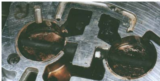
Picture J - Carburetor plates before P.i. treatment
