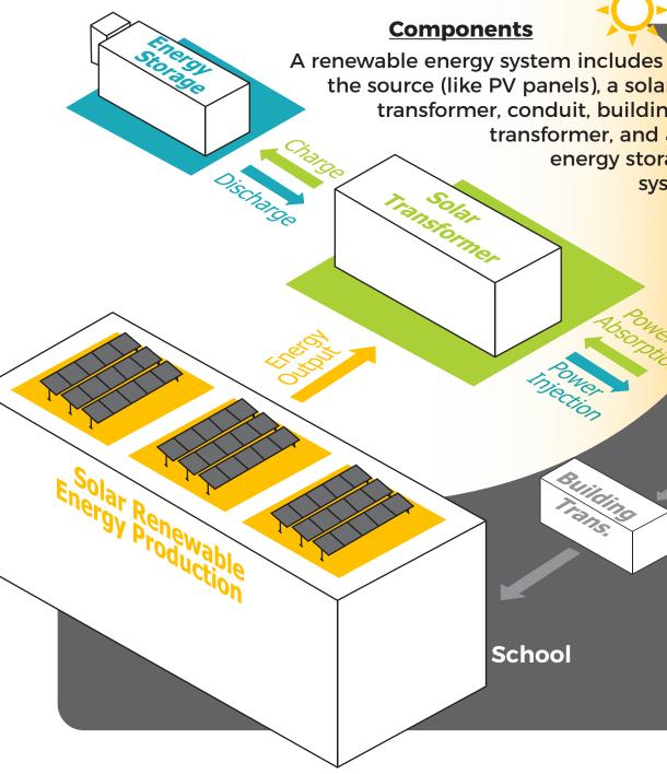
the source (like PV panels), a solar transformer, conduit, building transformer, and an energy storage system
