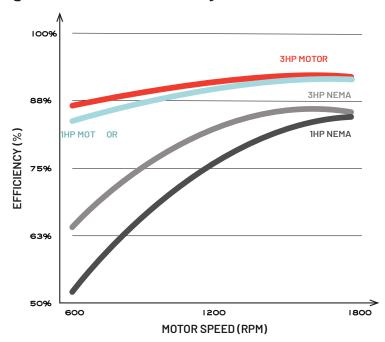
**QMC Quark** Motors exceed the efficiency of NEMA Premium Motors at all speeds.
