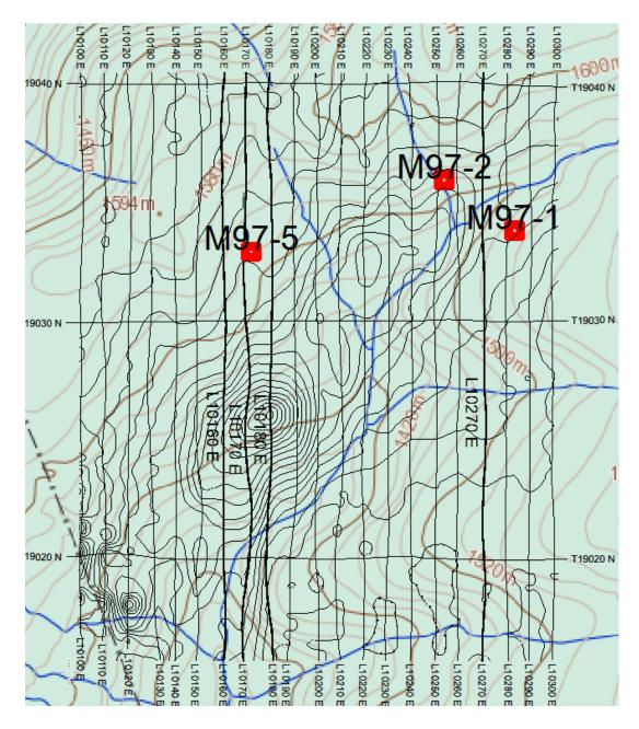
The resistivity low (high EM response) is due to a conductive surface layer. Contour lines are EM response/
