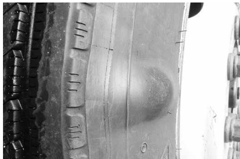
Sidewall Bulge Due to Impact with Pothole or Curb
