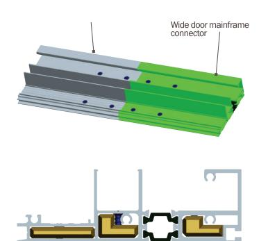
Mainframe and connector sectional view
