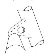
Assemble as shown to forks. Torque to 25-30 ft. lbs.
