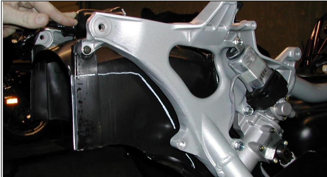
3. Drill the threads out of the two saddlebag/trunk stay frame mounting bosses on each side of frame with a 21/64 drill. (4 holes total)
