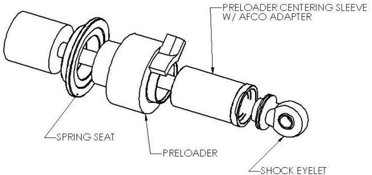
3. Remove the shock eyelet, jam nut, and shock preloader centering sleeve.
