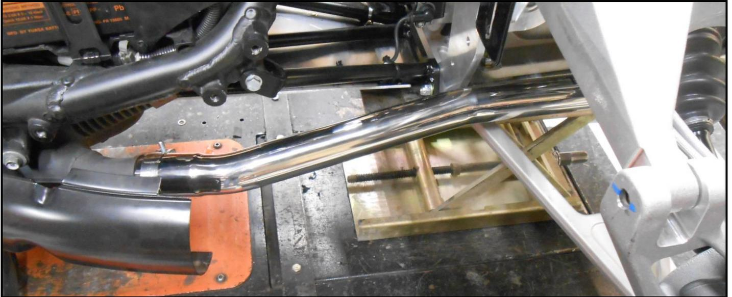
2. Install the 4 rubber sandwich mounts with flat washers and nyloc nuts to the Body Frame. Refer to **RED ARROWS**.
