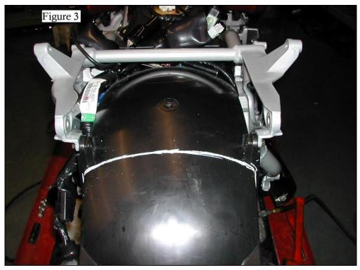
2. Using figure 4 as a guide, mark the outside of the inner fender to cut out the two sections for the intermediate mount.
