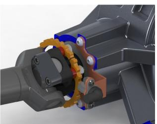
4. Place the driveshaft into the rear yoke and secure with two u bolts, lock washers and nuts.
