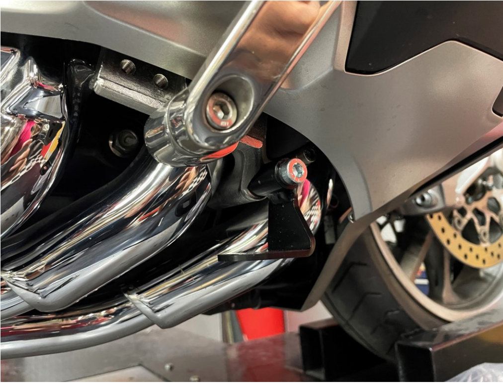
CSC GFX Mts installed with Goldstrike Peg Mts. Right Side
