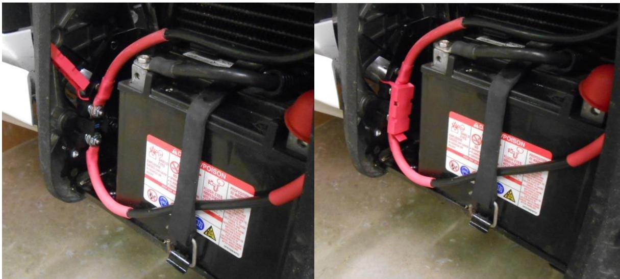
31. Install the short cable on the bottom post with a flat washer, cable, flat washer & nut.
