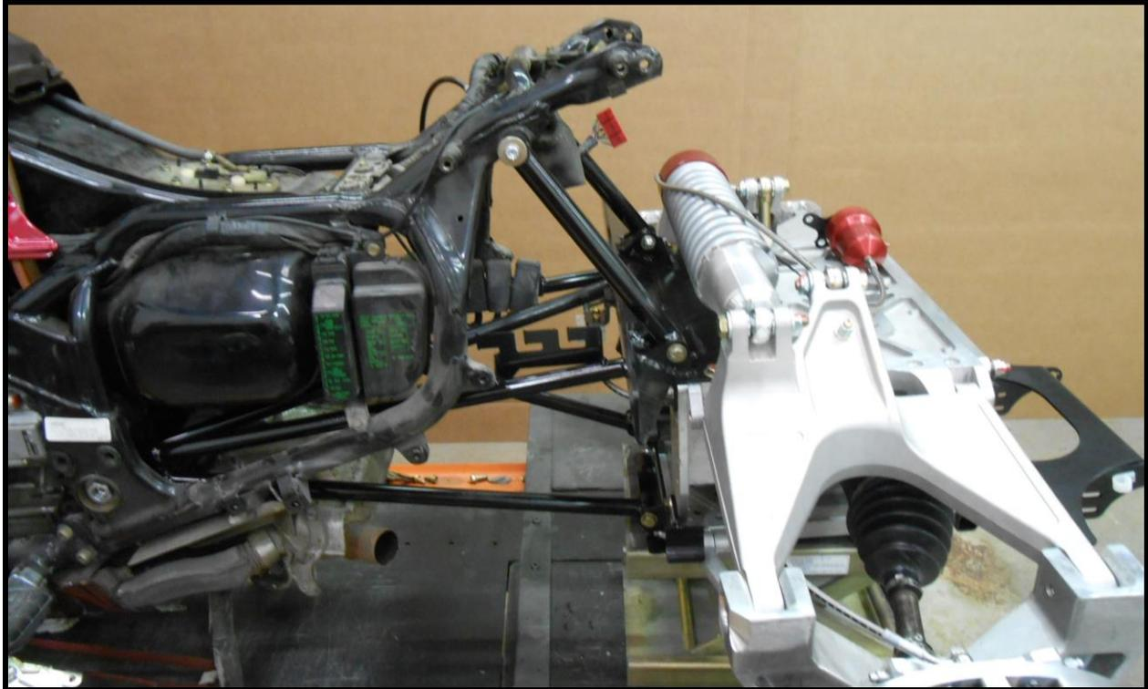
3. Moving the rear end forward. Align the frame mount bosses to the tabs on the lower front mount and the tabs on the intermediate mount.
