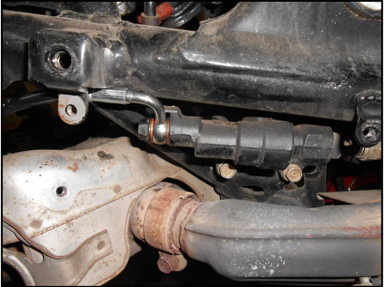
**34. Reinstall the rear brake master cylinder heat shields.**
