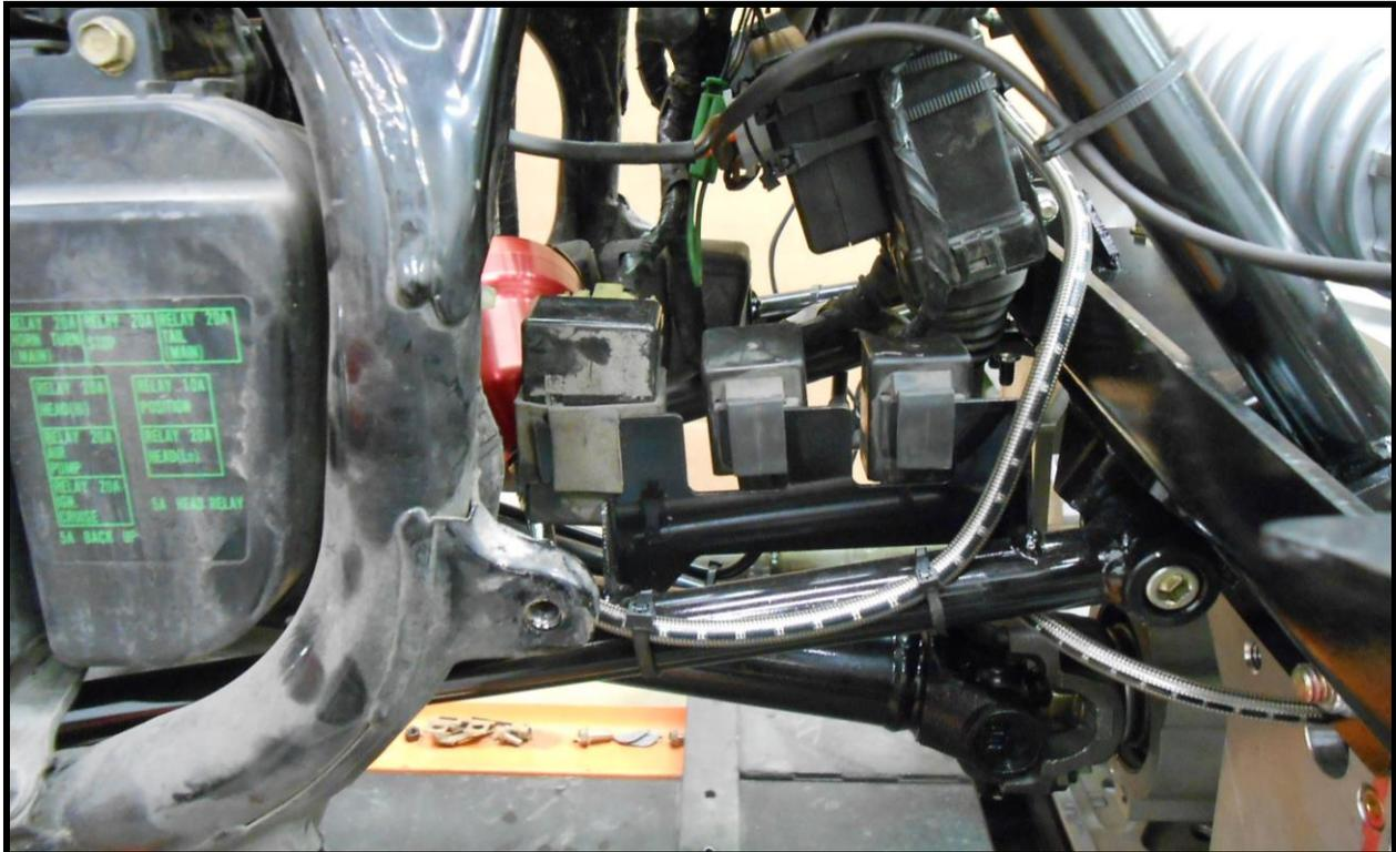
25. On the **GREEN** 3 pin connector for the Bank Angle Sensor connect the red and green wires together.
