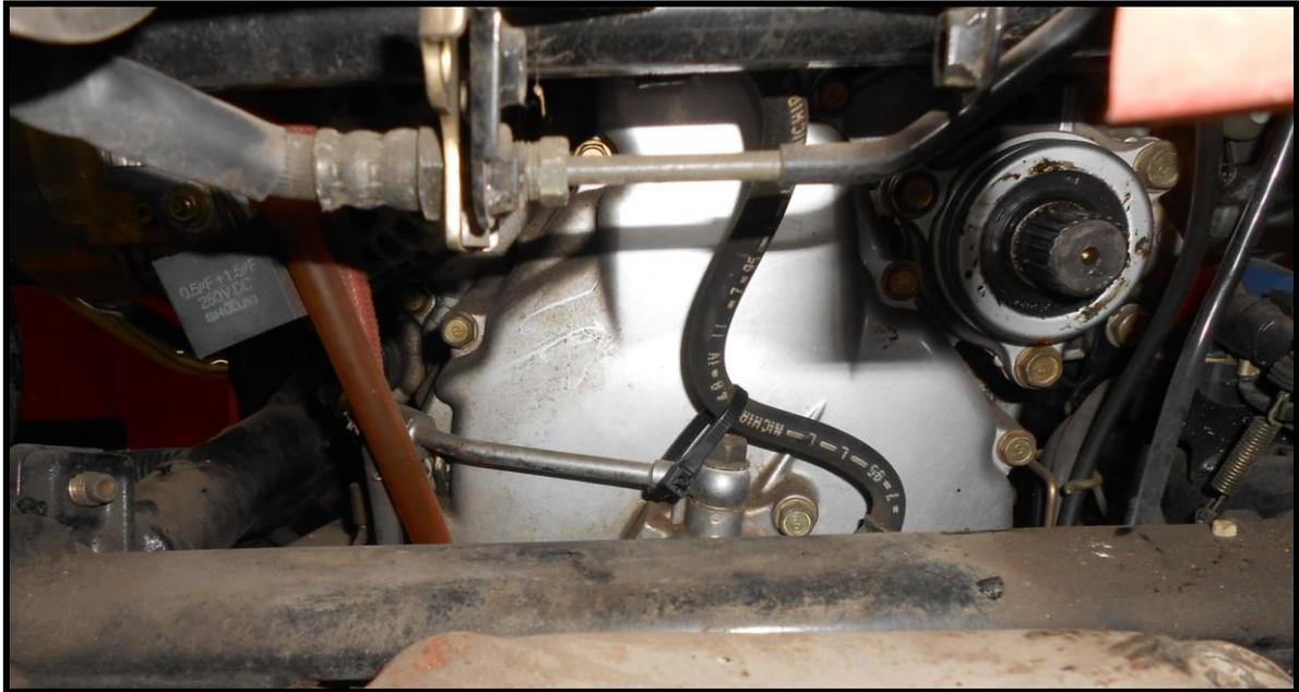
3. Bent down the left rear of the exhaust shield for mount clearance.
