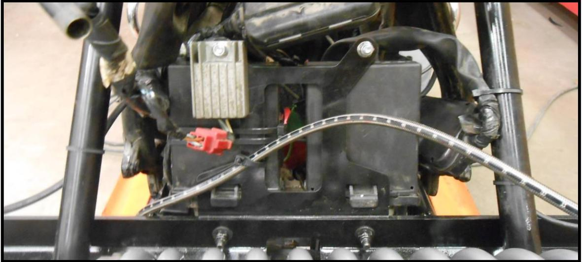
**29. If installing GRD EFX secure the GRD EFX control module to a control unit as shown.**
