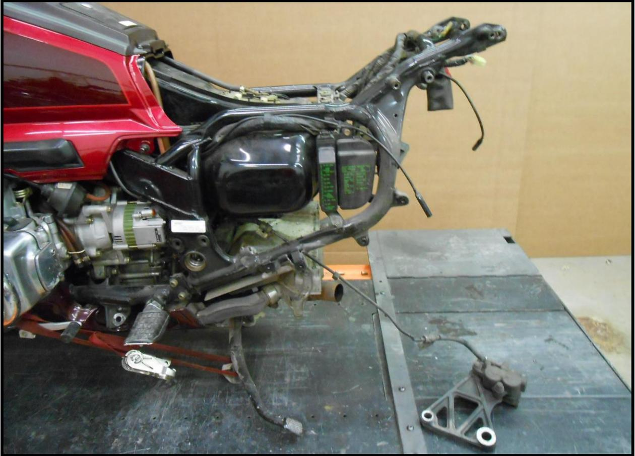
**28. Remove the ground wire bolt from the rear of the front inner rear fender. Unhook the 3 relays from the right side of the inner fender.**
