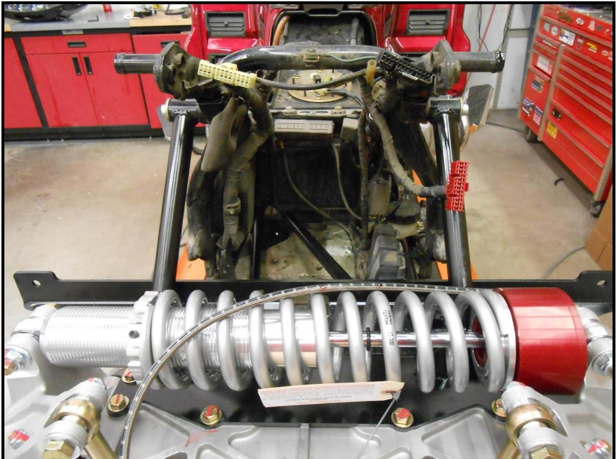
12. Secure with two **3/8-16 X 2 1/2 HHCS**, four flat washers and two nyloc nuts.
