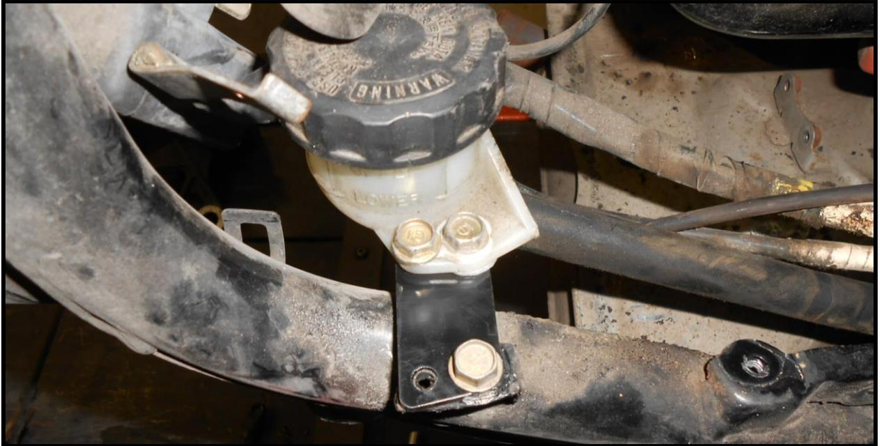
3. Position the right frame mount over the pivot bolt and route the master cylinder reservoir hose to the inside with the wire harness as shown.
