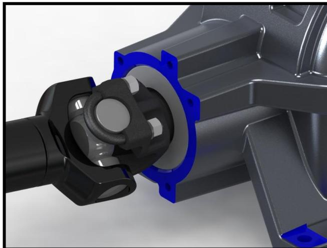
22. Tighten the four 3/8 HHCS and nyloc nuts that secure the differential to the lower suspension tray.
