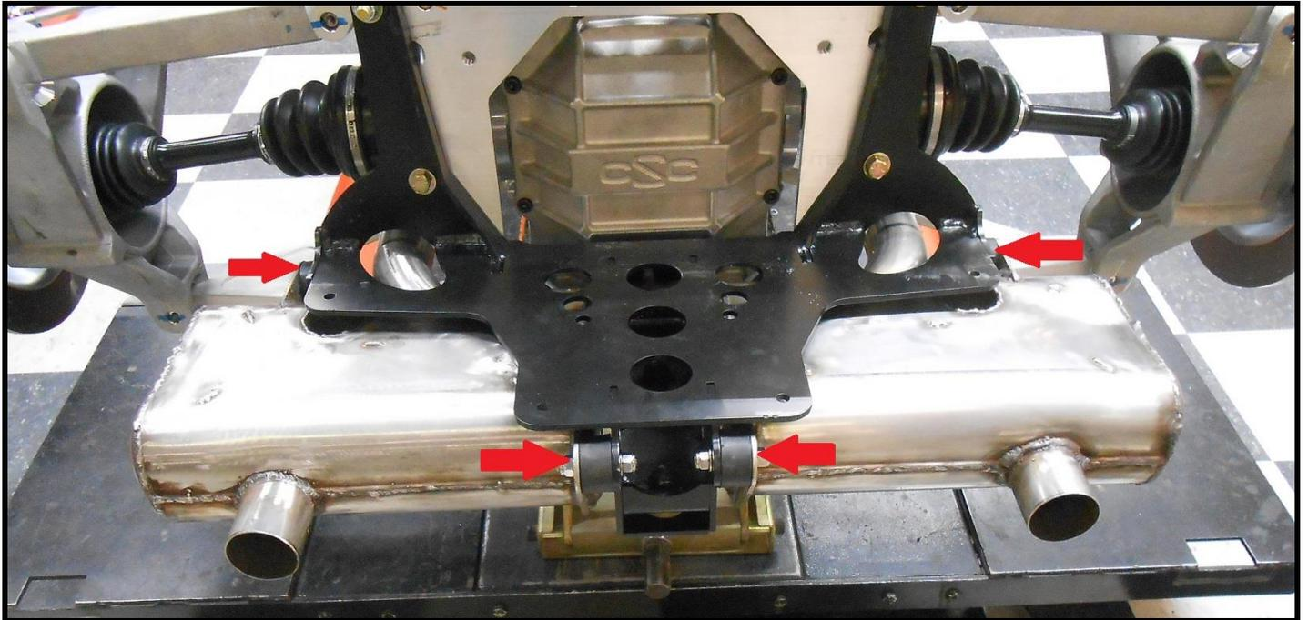
3. Slide 2 clamps on each side, 63 onto the rear of the tailpipes.
