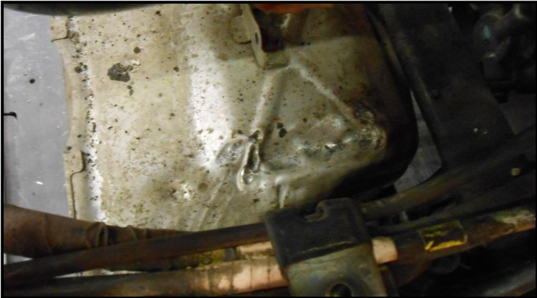
2. Secure the clutch hose to the left as far as possible for driveshaft clearance.
