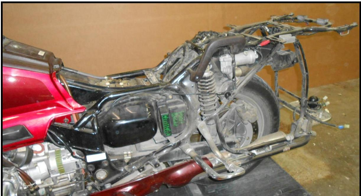
15. Remove and discard the mufflers, clamps and gaskets.
