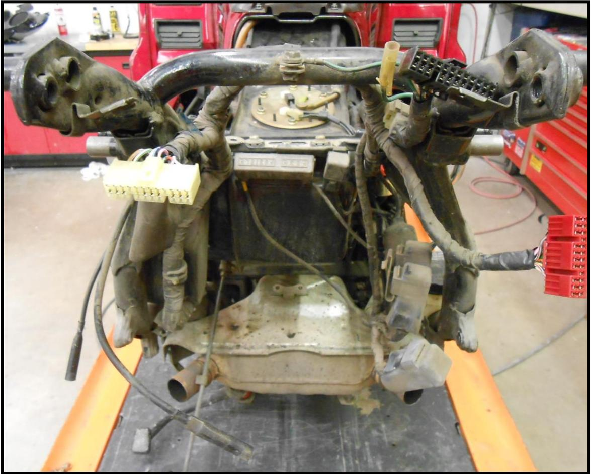
**30. Remove the rear brake master cylinder heat shields.**
