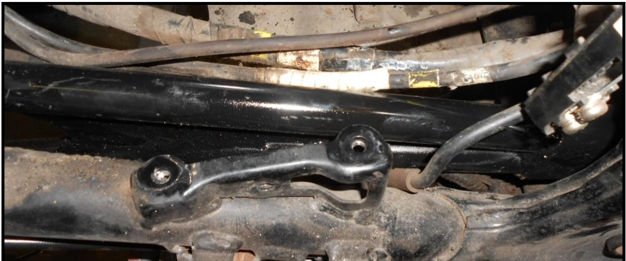
4. Loosely install a **3/8-16 X 1 3/4 SHCS** with thread locking agent into the frame mount threaded boss.
