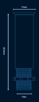
A small sized submersible stainless steel fitting with a countersink is the perfect accesory for water features, swimming pools and fountains.
