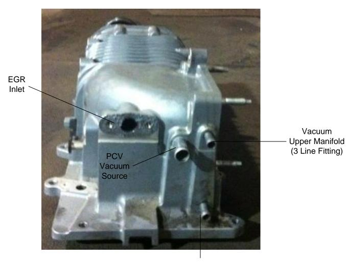
Vac/Boost Lower Manifold (2 Line Fitting)
