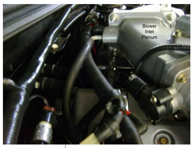
Hose To Evap System In Fender Rear Port
