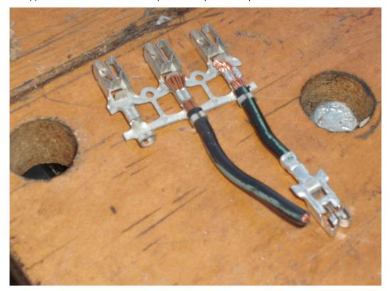
Insert the bus bar back into the rear of the fuse box and insert the new fuse connector into the available fuse slot:
