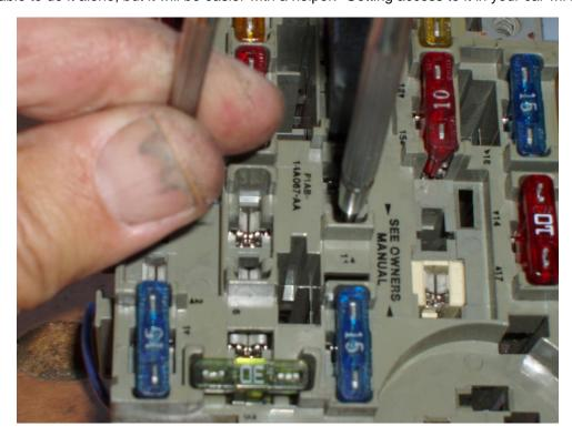
Here is the Fuse Bus Bar pulled out:
