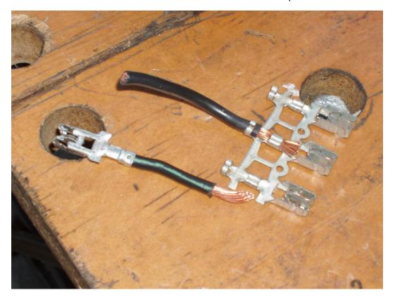
Now you will need to open one the unused crimps in the Fuse Bus Bar, using a jeweler's screwdriver. Select the unused crimp closest to the spare fuse location:
