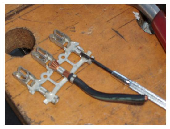
Insert the stripped end of the wire into the opened crimp and crimp the bus bar to the wire and the insulation:
