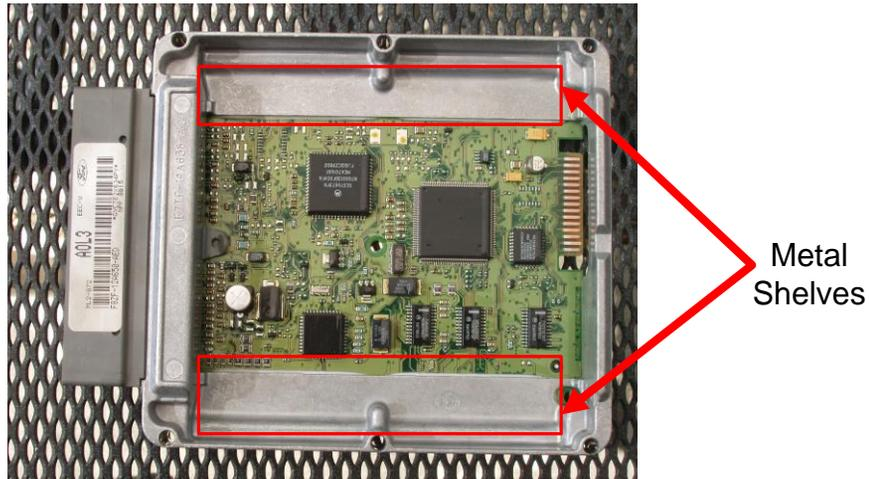
The metal shelves act as support for the PCB as well as a heat sink to the outside of the case. You can see the heat sink compound squeezing out from between the PCB and the shelves.
