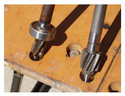
We emailed Quaife about the keeper and they said they had never been asked about it before. They suggested using a circlip if we were concerned about it. We measured the pinion shaft to be 15mm in diameter, and the keeper slot to be 13mm in diameter. But we weren't able to find a metric circlip, so we bought a ½" circlip because it was close, although a little too small. We used a compass to draw a 13mm circle, and laid the circlip on it to see how much of the inner prongs needed to be cut:
