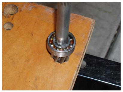
We pulled out the rack end bushing and applied a thin layer of grease to the inside. Be careful not to clog the air channels with grease because air needs to flow through the bushing.
