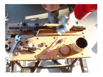
With a Dremel tool with a cutoff wheel, we cut the bearing keeper off of the stock pinion shaft, and drove the bearing off of the pinion. We cut the center out of the bearing to get the stock bearing race. We used the bearing race with a hammer to drive the pinion and bearing into the gearbox housing:
