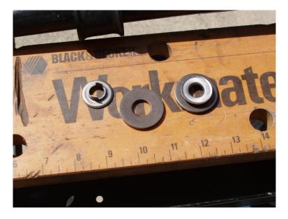
And how they go on each end of the rack. Make sure the tabs in the lock washers slide into the slots on the rack ends::
