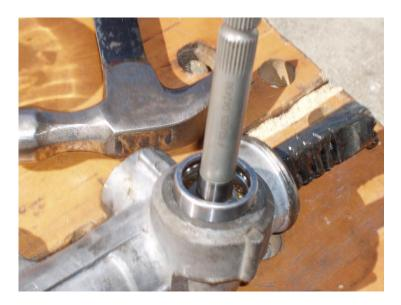
We replaced the internal 35mm snap ring:
