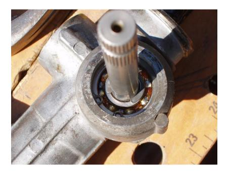
We greased the pinion dust seal, and used the old pinion bearing race and a hammer to tap the dust seal into place:
