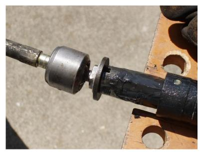
Using a chisel and a punch, flatten the lock washers against the flat sides of the tie-rods:
