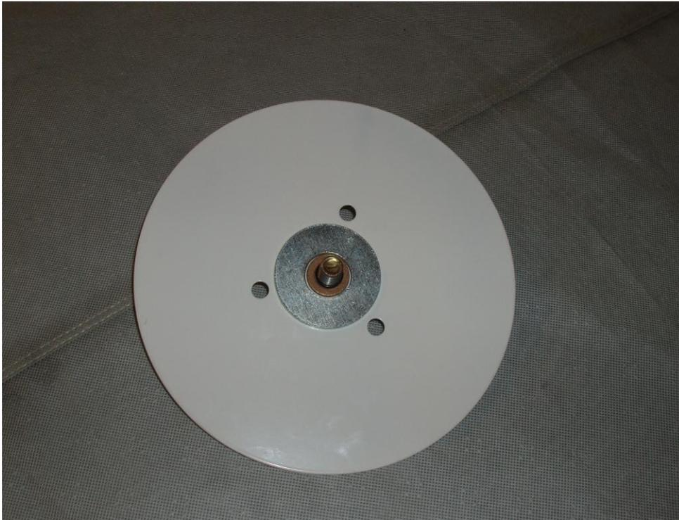
Hold the large flat washer against the back of the degree wheel with two fingers while you screw the crank bolt into the crankshaft. Make sure that the larger washer stays around the OD of the bronze bearing, so it can clamp the degree wheel:
