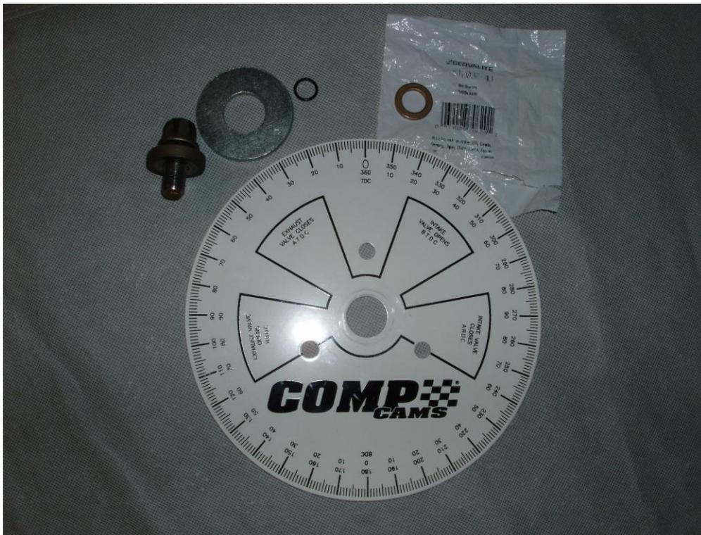
The Servalite bronze bearing is the key item because it fits perfectly inside of the Comp Cams Degree Wheel and almost perfectly around the stock crank pulley bolt. I found it in the Hard-to-find section of the hardware store. Unfortunately, it is a bit thicker than the degree wheel, so the large flat washer is required to clamp the degree wheel in place against the end of the crankshaft.
