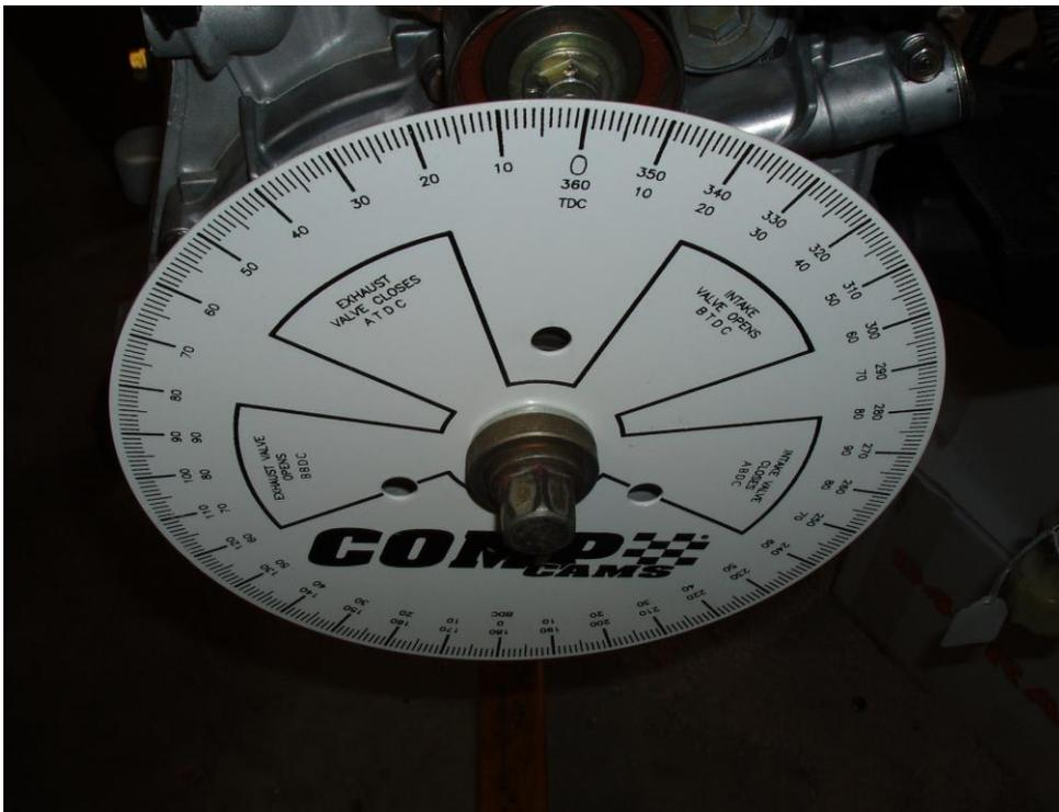
The only downside of this setup is that the B-series engine rotates counter-clockwise from the crank side, so you can't use the crank bolt to rotate the engine during the degreing process since it will come loose. You will need to rotate the engine using the flywheel during the degreing process.
