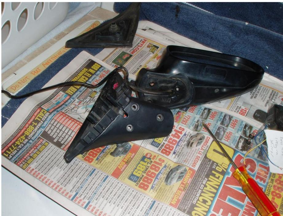
I washed the mirror body and used Meguiar's Dash & Trim Restorer on it. It came out nicely. The mirror base paint was starting to oxidize a bit, so I used Meguiar's Finish Restorer first, followed by their paint cleaner, and finally with a coat of their wax. Here is a picture of the passenger mirror base after cleanup next to the driver mirror base as it came from the junkyard:
