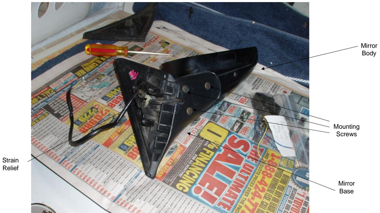
Make a drawing of the connector pinout (you will need to put it back the same way) and then de-pin the connector, and remove the 4 screws. Here are my mirror side connector pinouts from the pin side of the mirror connector:
