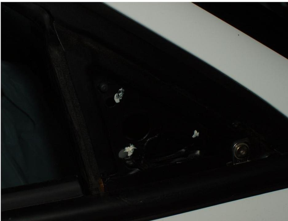
It took a lot of grinding to get slot the holes far enough to mount the mirrors to the doors. Also, it took longer screws. It turns out that sunvisor screws work perfectly. Here is the mirror installed on the CRX:
