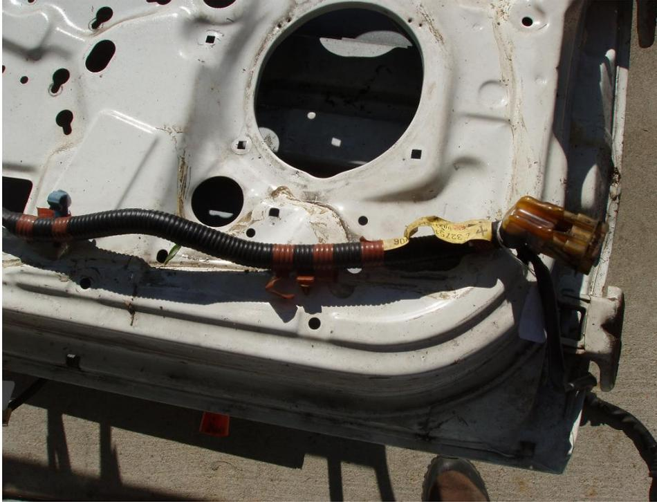
Here is the harness installed with the connector in the door.
