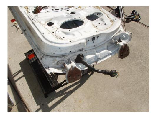
Hold the harness against the wire harness clip holes and mark the harness so you will know where to mount the clips. I used White-out to mark the harness.
