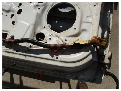
Here is the harness installed with the connector in the door.
