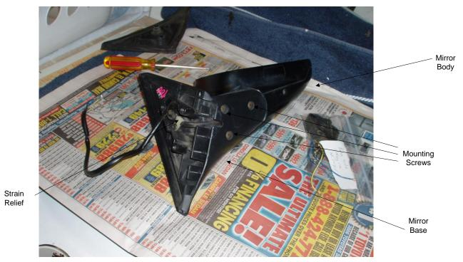
Make a drawing of the connector pinout (you will need to put it back the same way) an then de-pin the connector, and remove the 4 screws. Here are my mirror side connector pinouts from the pin side of the mirror connector:
