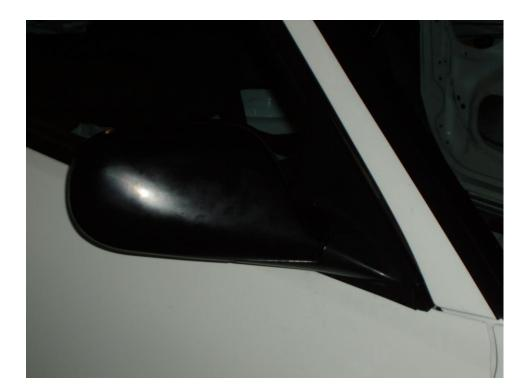
The Integra mirror leading edge has a slight curve to it vs. a straight line on the door frame, but it is barely noticeable. When you test fit everything, you will see how far you need to extend the mirror wires to reach the connector on the door harness. Extend the wire, re-pin the connector and plug in the extended wires and you are done. We will be making interior mirror lever block-off plates later to finish the internal trim.
