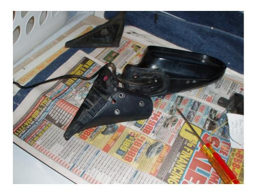
I washed the mirror body and used Meguiar's Dash & Trim Restorer on it. It came out nicely. The mirror base paint was starting to oxidize a bit, so I used Meguiar's Finish Restorer first, followed by their paint cleaner, and finally with a coat of their wax. Here is a picture of the passenger mirror base after cleanup next to the driver mirror base as it came from the junkyard:
