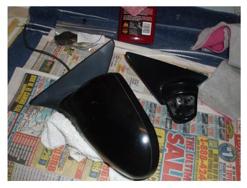
Reinstall the mirror body to the base using the three screws. I noticed that they had some kind of thread-locker on them, so I reinstalled ours with blue Loctite. Reinstall the strain reliever on the wire. We reused the CRX mirror gasket. If you stretch it a bit, it will fit. I used some shrink tubing to seal the wire sheath to the mirror gasket, rather than the black tape that Honda used:
