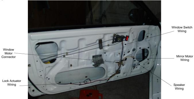
The following pages show the stock wiring of the 4 door Civic Window followed by the modified wiring. The speaker wiring needs no modification, nor does the mirror wiring other than extending the wire from the mirror.
