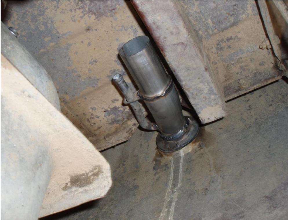
We then slid the Unicoil over the 1/2" fuel rated hose, and bent the 90 degree angle into it. We fit it to the fuel tank, cut the length to fit the nipple on the filler neck vent pipe, and installed it.
