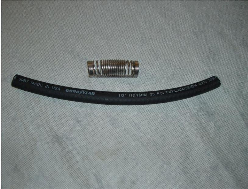
The Unicoil allows you to make a sharp 90 degree bend in a hose without causing the hose to crimp itself closed.
